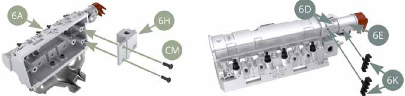
Connect one end of 6J High tension lead to pointed 6A Spark Plug and the other end to pointed 6G Distributor cap contact. Fit loose stretch of 6J High tension lead to lowest slots of 6K Lead guides. Connect one end of 6J High tension lead to pointed 6A Spark Plug and the other end to pointed 6G Distributor cap contact. Fit loose stretch of 6J High tension lead to next higher slot of 6K Lead guides.
