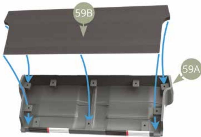
Fit 59C Backrest inner panel on top of 59B Backrest padding well into 59A Rear seat backrest and same way under its ten perimeter tabs.
