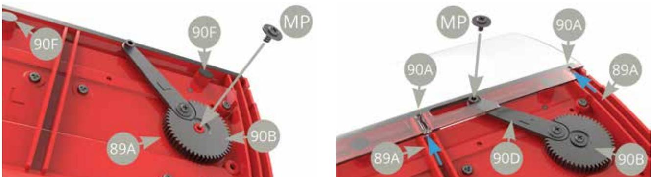
Fit 90C Small gear to 89A Left door inner panel peg,engaging (meshing / INTERLOCKING) it with 90B Big gear (90A Glass raised up). Make sure to adjust the raised sector edge (green arrow) being in front of blue arrow pointed edge, and then fix 90C Small gear to 89A Left door inner panel with MP screw. Peel two 90F Protective roundels off backing paper and stick to 86A Left door protrusions on its inner side.
