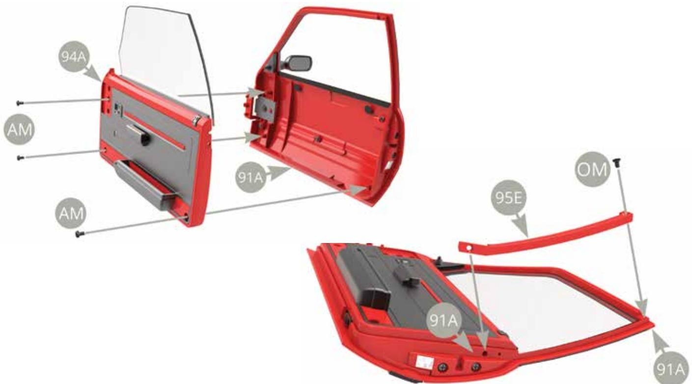
Fix 91A Right door to 94A Right door inner panel with AP screw. Fix the other end of 95E Plank to 91A Right door with OM screw. Rotate 95C Small gear (blue arrow) with your finger to check lowering and raising 95A Right door glass (green arrow).
