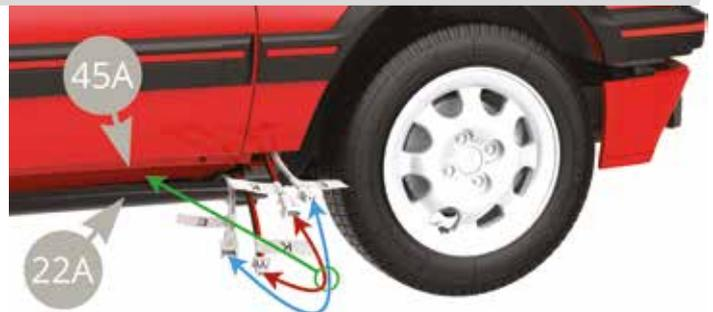
Once all the wiring is correctly placed in its slots, fully engage 64A (body) to the 22A (chassis) - blue and red arrows in the illustrations below.
