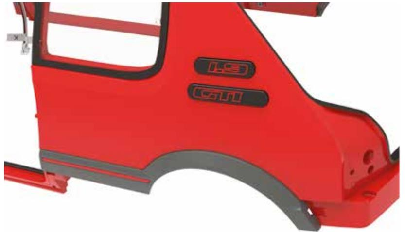
Fit 75C Right GTI molding and 75D Right L9 molding to 64A Body.
