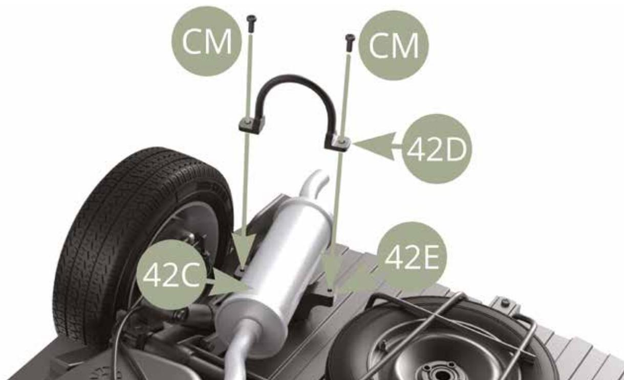
Fit 42C Exhaust silencer to 42E Exhaust mount and secure it with 42D Clip and two CM screws (bottom illustrations).
