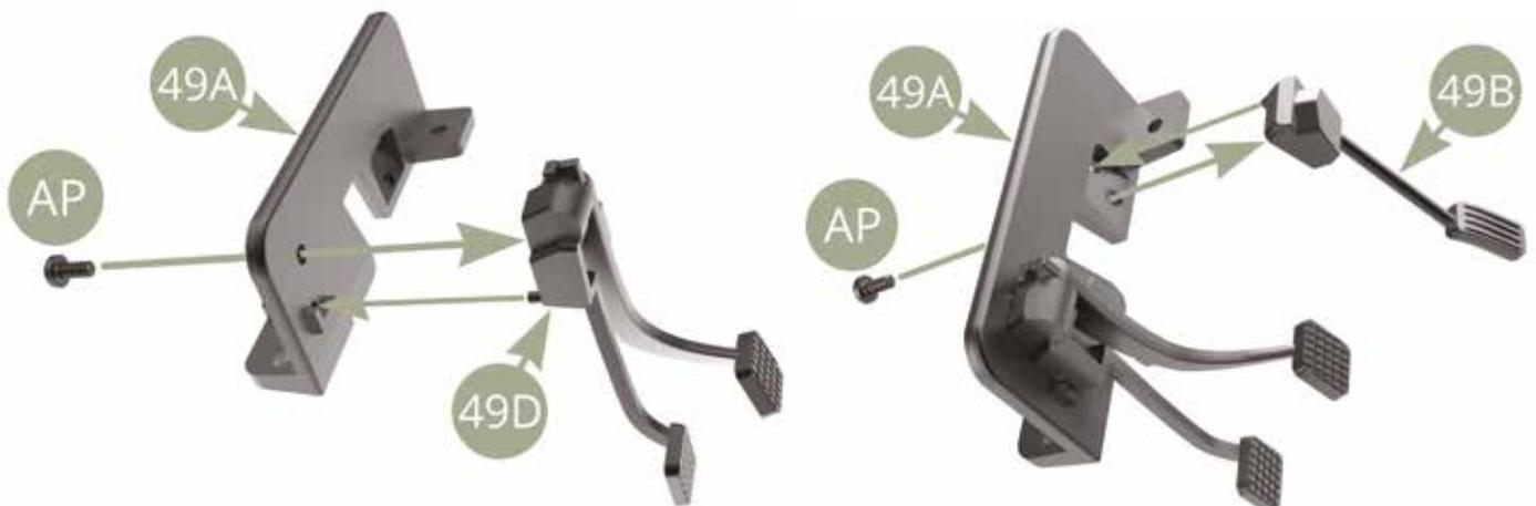
Fit 49A Pedal's panel to 45A Cabin floor pin (blue arrow) and fix with AP screw.
