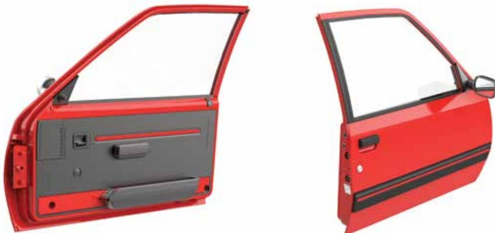
Fitting the Right door to the Bodywork, aim 92H Hinge pins to fit into the sockets on 64A Body frame (green arrow), and 91A Right door inner upper corner to push up 66G Switch lever (blue arrow). Refer to upper and lower illustrations.
