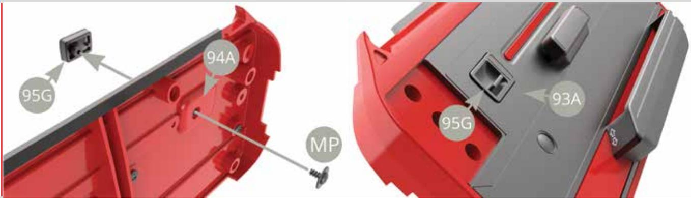
Peel two 95F Protective roundels off backing paper and stick to 94A Right door inner panel protrusions, to keep door glass from scratching during its movement. Fit 95D Lever to 95B Big gear and fix with MP screw.
