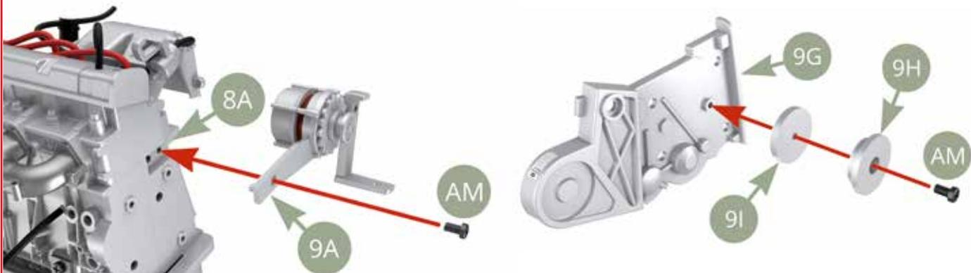
Fit 9J Engine mount to 9G Timing belt cover and fix with BM screw. Fit 9G Timing belt cover to 8A Left and 8F Right Engine blocks and fix with four AM screws.
