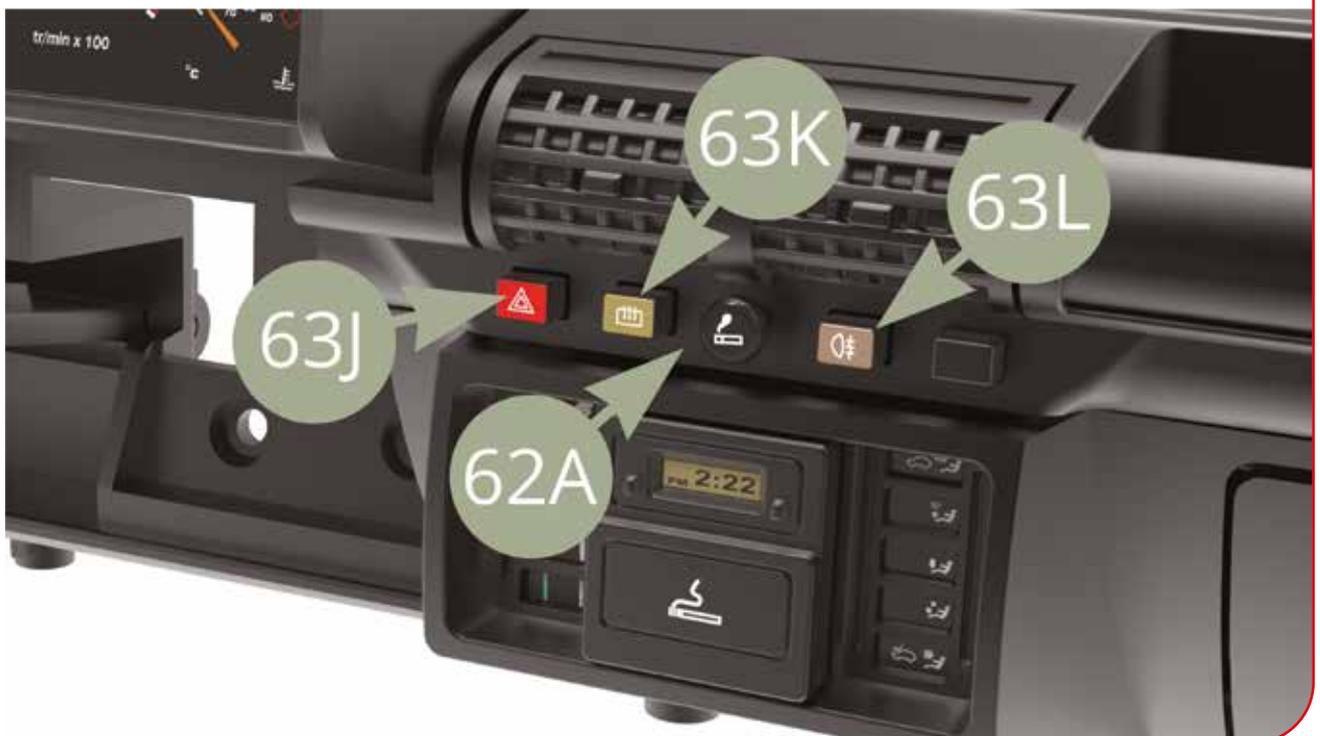
Aim to fit switches of 63N G Cable (white-gray), 63O M Cable (green-yellow) and 63P S Cable (red-green) into sockets of 63J Hazard warning, 63K Rear screen heater and 63L Rear fog lamp buttons, securing 63I Switch holder to 62A Facia panel back side with two AP screws (top and bottom illustrations).
