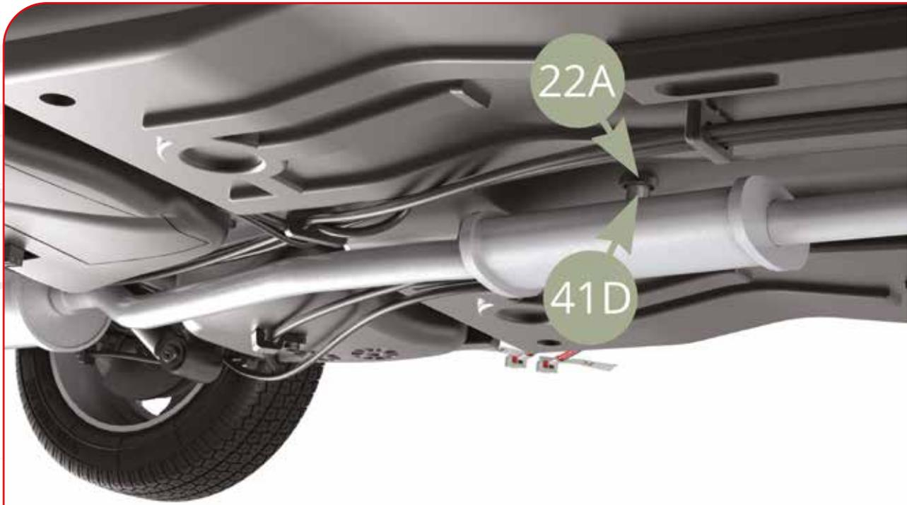
Fit 41D Catalytic converter top peg into 22A Chassis panel nest and fix from above with IP screw (bottom illustrations).
