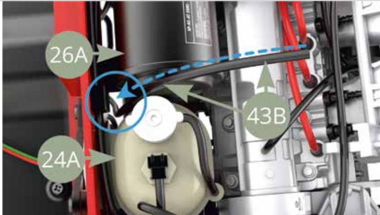
Turn chassis over and continue to lead 43B Fuel return pipe vis three 23B Clamps leaving the end loose.
