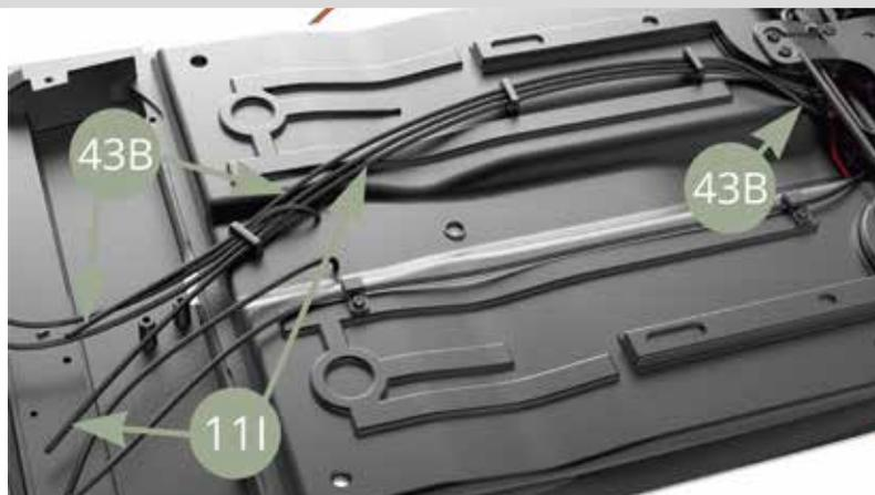
Turn the chassis back on wheels, and fit 43B Fuel return pipe to 7E Fuel injection rail stub-pipe.
