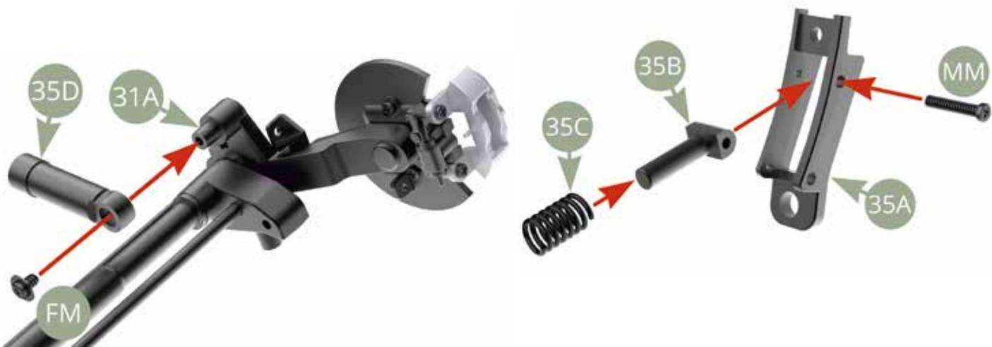
Fit 35B shock absorber piston into 35D Shock absorber cylinder and then, fit 35A Rear axle left base end on 33A Rear axle left mount pin (illustrations below).
