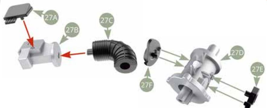
Fit 27D Throttle body to 27C Air duct.
