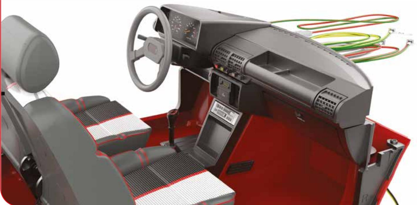
Guide 63N G Cable (white-gray), 63O M Cable (greenyellow), 63P S Cable (red-green) and 61F J Cable (redgreen) between two pegs on 48A Centre console, secure them with 63M Clamp and fix with AP screw.
