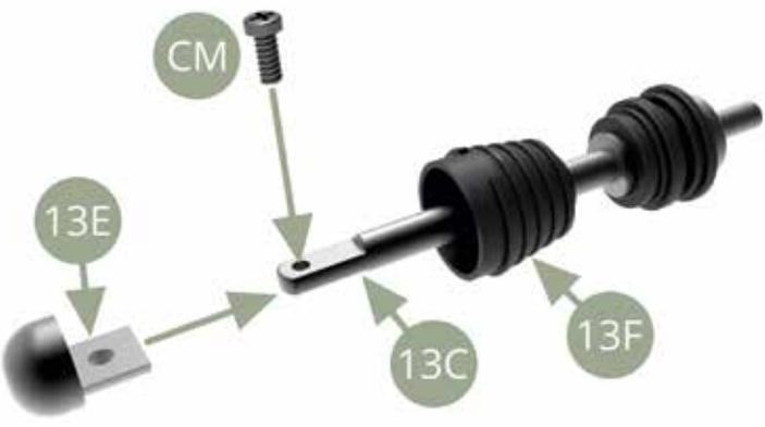
Slide 13F Rubber bellows along 13C Driveshaft to cover the joint (blue arrows motion).
