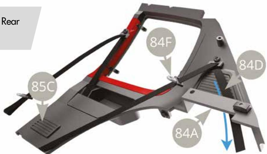
Pull to tighten the upper end of 84D Rear right safety belt (blue arrow). Lead 80C Cable along 80A Ceiling panel edge to exit where green arrow point. Fit 85D Parcel tray left side peg into the socket on 82A Interior left panel, holding it suspended.
