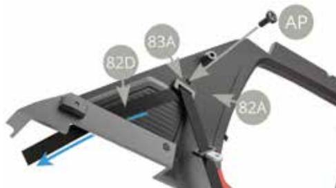
Wrap the other end of 82D Rear left safety belt over the notch in lower edge of 82A Interior left panel (upper illustration, blue arrow) and fix it (punching with thick needle or awl, red arrow, lower illustration) with AP screw, attaching 83E Deco grid panel at the same time. Note 83B Buckle position on upper illustration.
