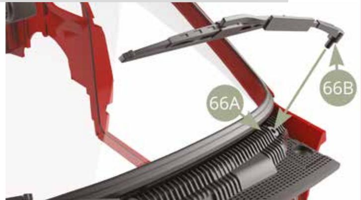
66D+66E Right and 66B+66C Left Windscreen Wipers are installed on 66A Air intake grille.
