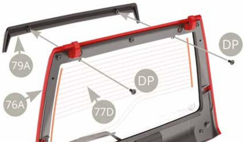
Fit DP screw to upper right corner of 78A Tailgate inner panel, leaving space under screw head to loop over and tie to knot first 79F Rear shelf support rope (lower illustrations).
