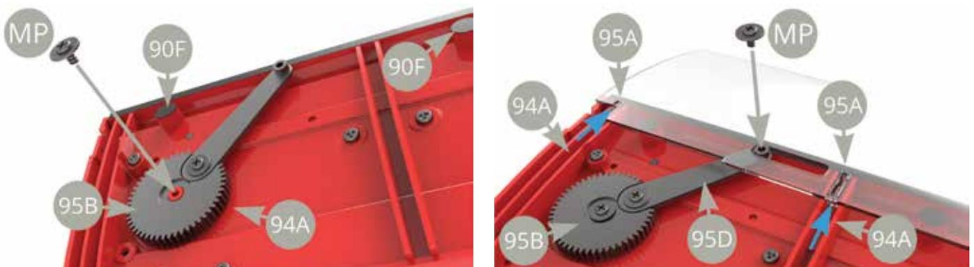
Fit 95C Small gear to 94A Right door inner panel peg, engaging (meshing) it with 95B Big gear (95A Glass raised up). -Make sure to adjust the raised sector edge (green arrow) to be in front of blue arrow pointed edge, and then fix 95C Small gear to 94A Right door inner panel with MP screw. Peel two 95F Protective roundels off backing paper and stick to 91A Right door protrusions on its inner side.
