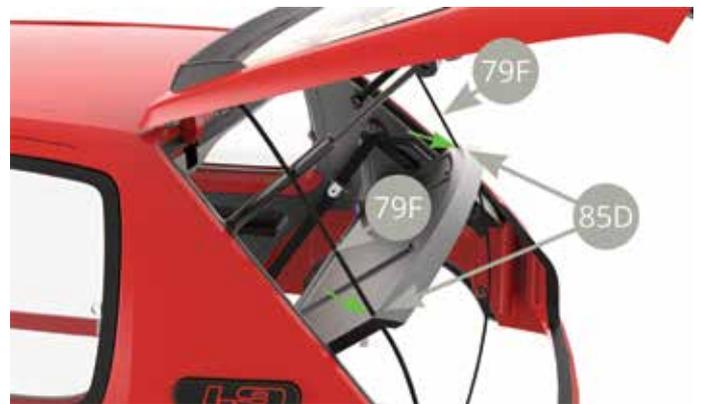
Close the Tailgate, upturn the car body, pull 79F Parcel tray support cords to tighten them, with 85D Parcel tray itself in its stowed (horizontal) position. Tie 79F Cords to knots close to 85D Parcel tray surface (blue arrows). Upturn car body again, open the Tailgate, the 85D Parcel tray will lift up, pulled by 79F Cords. Cut excess lengths of 79F Cords some 5mm lower from the knots (green arrows).
