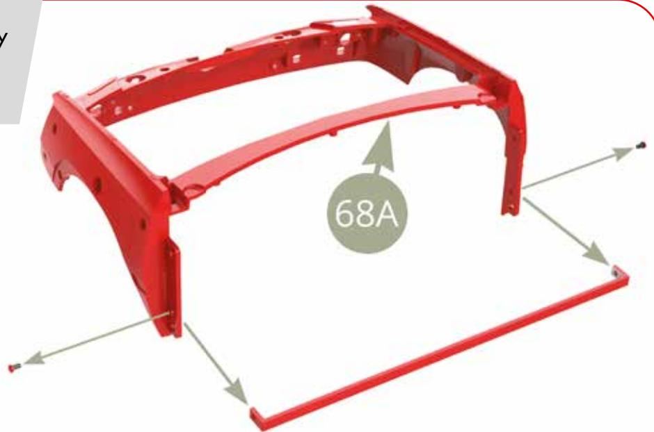
To facilitate further assembly cut the threads by taking four GM screws and screw them in (blue arrows) 68A Front subframe right (upper image) and left (lower image) side flanges, and then unscrew completely (red arrows).
