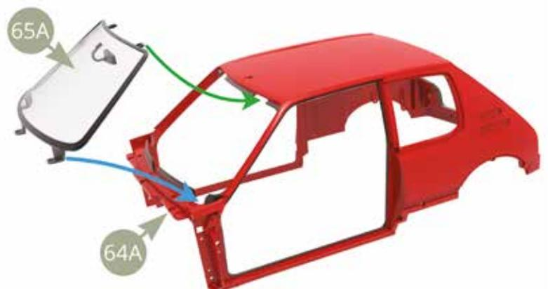
Fix three lower tabs of 65A Windscreen to 64A Body frame with three AM screws.
