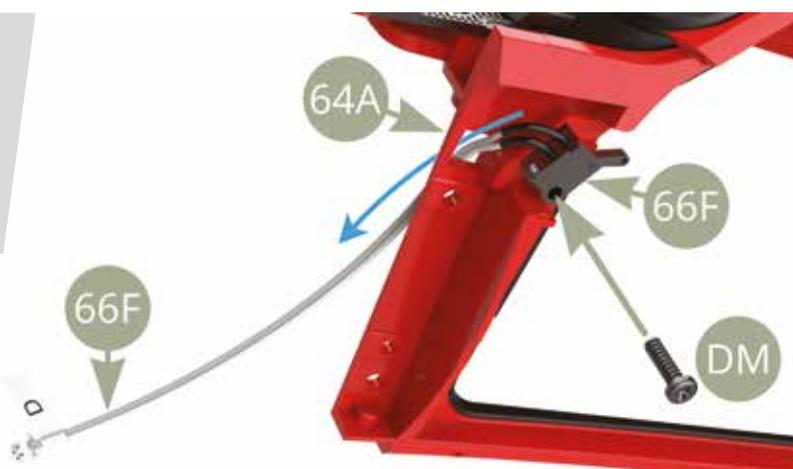
Fit 66G Saloon light switch cable E through square opening on the right side of 64A Body frame (blue arrow) and fix the switch with DM screw.
