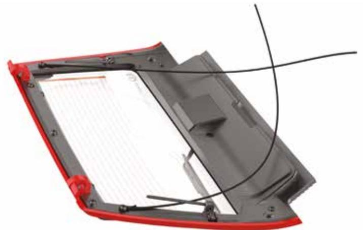
Fit 76A Tailgate to 64A Body frame rear opening, fitting 76B Left and 76C Right tailgate hinge axles into respective grooves in 64A Body frame inner ceiling edge (lower illustrations).
