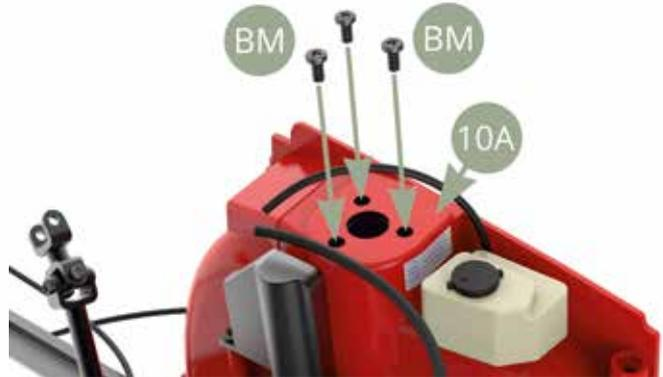
Fit 15A Top mounting to 10A Front wheel arc frame and fix with three BM screws (illustration above and below).
