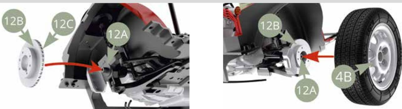
Fix 4B Wheel rim hub with KM screw via 4D Washer. Keep 4C Hub cover in safe place for later assembly stages.
