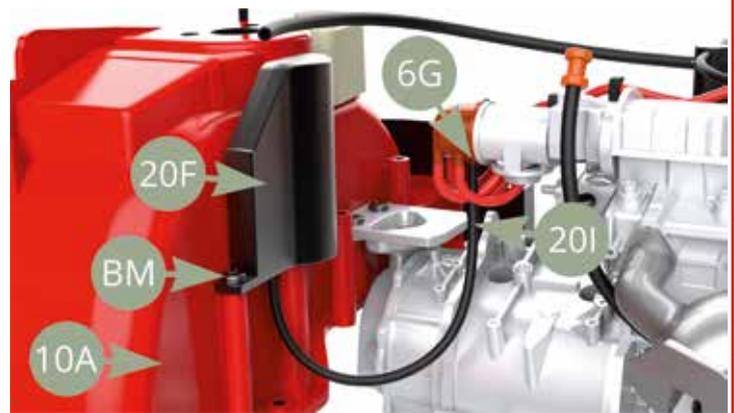
20I High tension lead connected to 6G Distributor cap.
