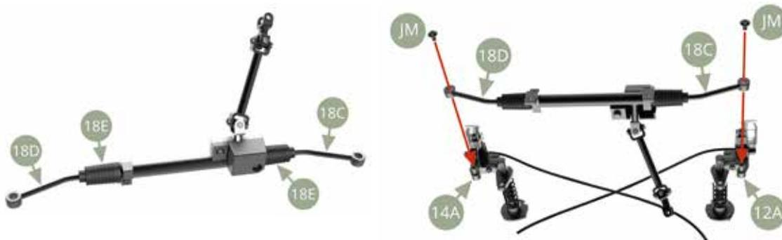
Fit 17B Steering column to 16B Subframe and fix with two BM screws. At the same time, guide two 18F Link arms to fit 12F and 14F Front suspension struts.
