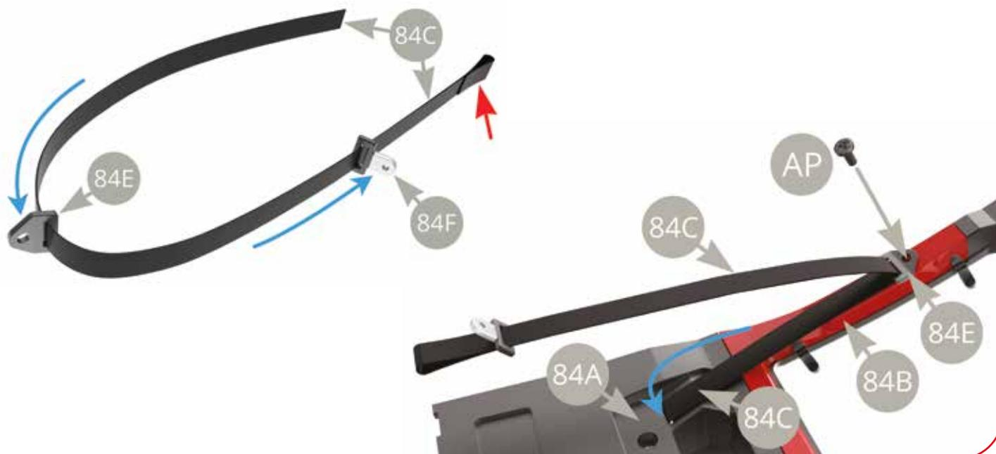
Tie a knot (red arrow) at approximately 15mm distance from 84C Front right safety belt end, to serve as stopper. Pull 84C Front right safety belt as blue and green arrows point, to position the belt.
