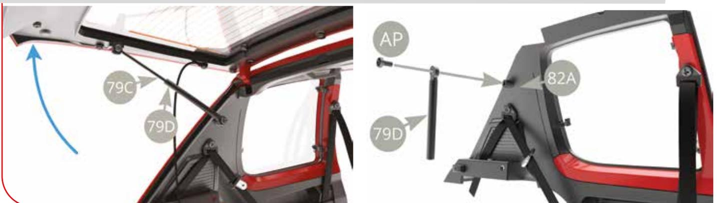
Check 79D Tailgate strut with closed Tailgate. Pull to tighten 82D Rear left safety belt (blue arrow).
