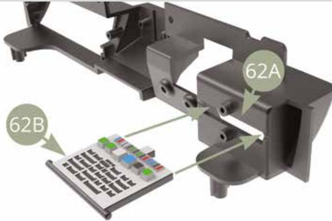
Fit 62C Clamp to 62A Facia panel, securing 62B Fuse console, and fix with two AP screws.
