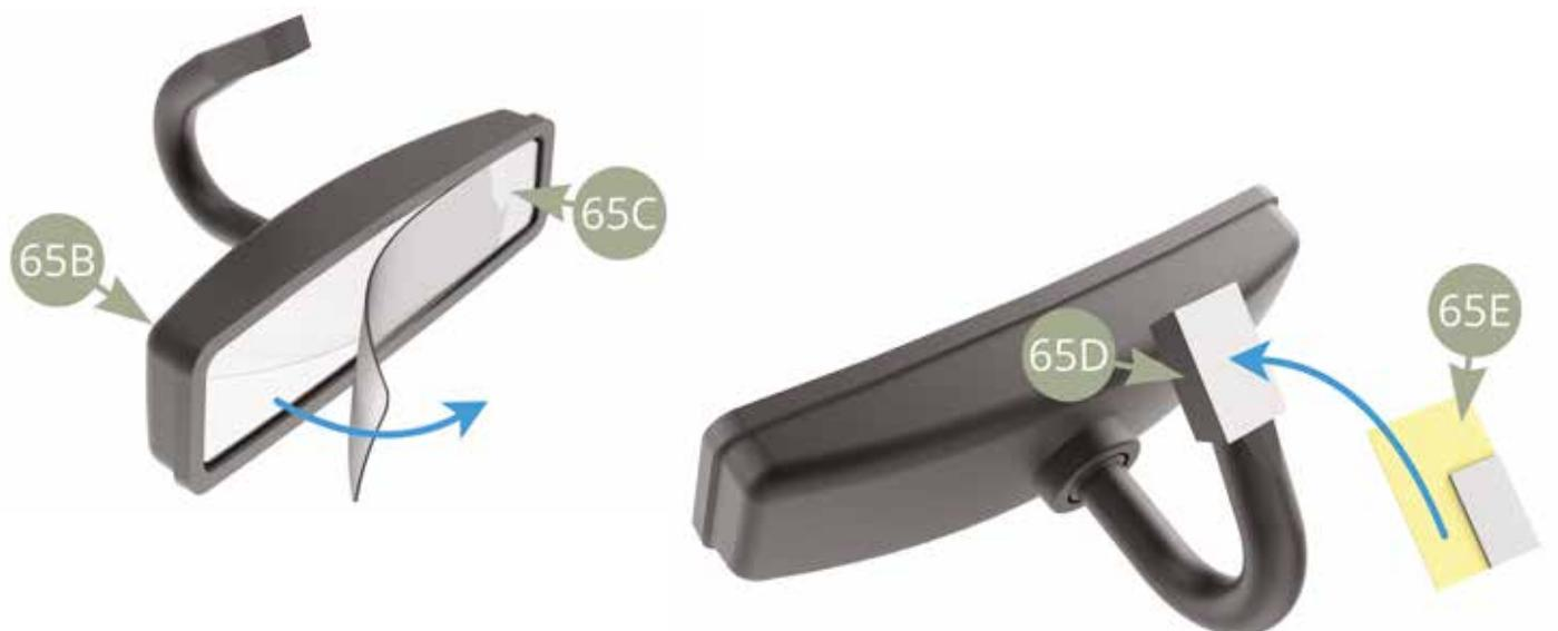
Peel away (blue arrow) 65E Double side tape white backing paper leaving sticky transparent tape attached to 65D Rear-view mirror arm (red arrow).
