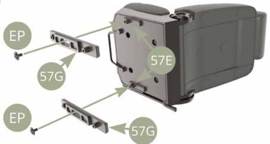
Adjust EP screws tension to allow 57G Rails slide motion (red arrows).
