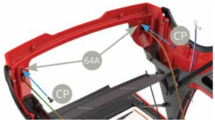
Lead right side 96E H cable along 64A Bodywork side and together with 80C F cable fix by 96F Tape piece. Lead left side 96E H cable along 64A Bodywork side and fix by 96F Tape piece.
