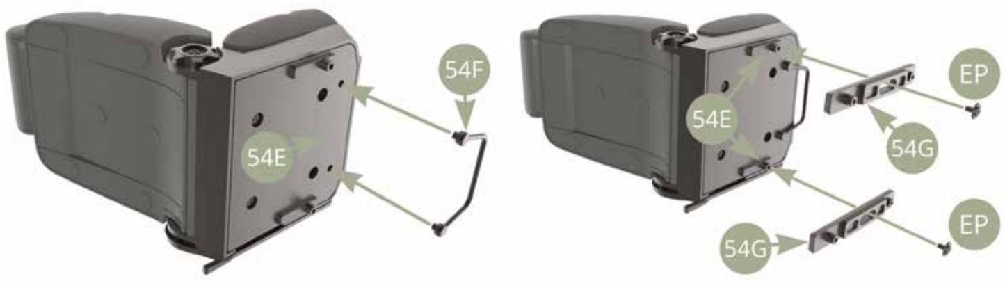
Adjust EP screws tension to allow 54G Rails slide motion (red arrows).
