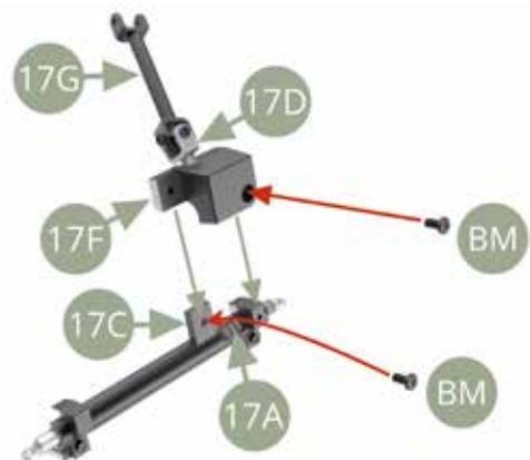
The resulting Steering Gear assembly should have 17A Steering rack both ends exiting approximately same distance from 17C Steering column in neutral / centered position. Rotate 17G Intermediate shaft left / right to check respective 17A Steering rack movement function.
