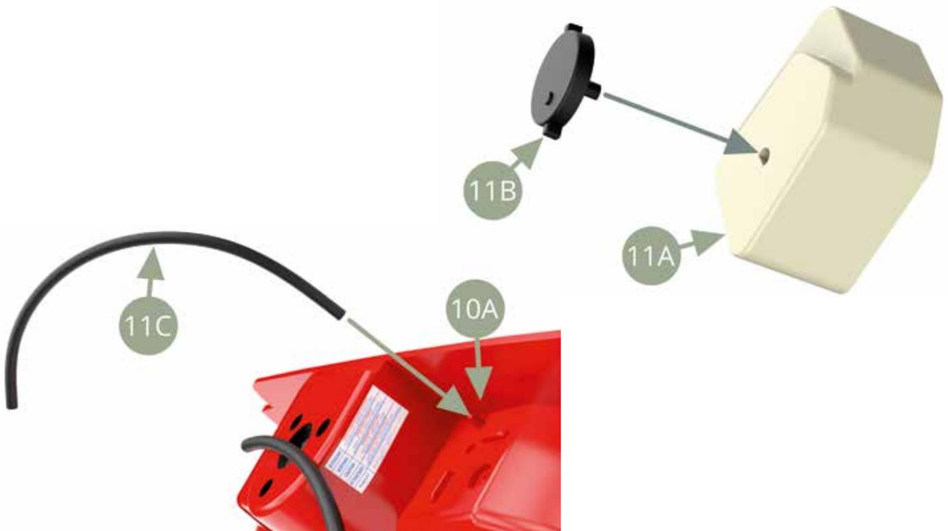
Fit 11A Washer fluid reservoir to 10A Front wheel arc frame and fix with CP screw from below (follow bottom illustrations).
