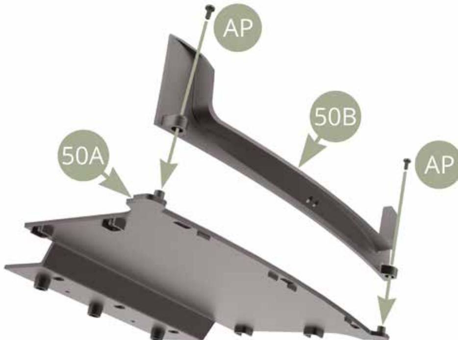
Fit 50D Trunk left panel to 50A Trunk floor and fix with two AP screws.
