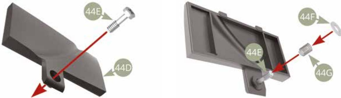
44G Pop up spring and 44F Washer fitted to 44E Battery cover lock screw.
