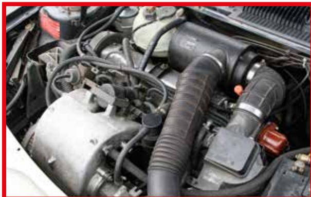
*The 1.9-litre engine is based on the previous XU5 J-type four-cylinder, but with a 15mm longer stroke. It is mated to a BE3/5-type gearbox that is remarkably well-calibrated and easy to handle.*
