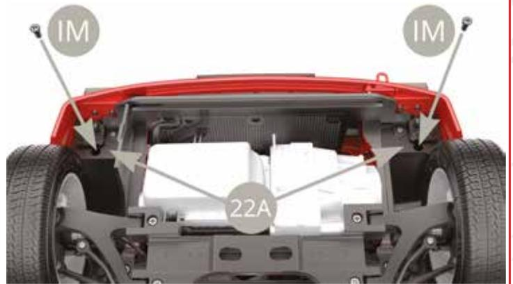
Complete the installation of the 22A chassis with two IM screws on the rear part of the car. Turn the switch to OFF (red arrow).
