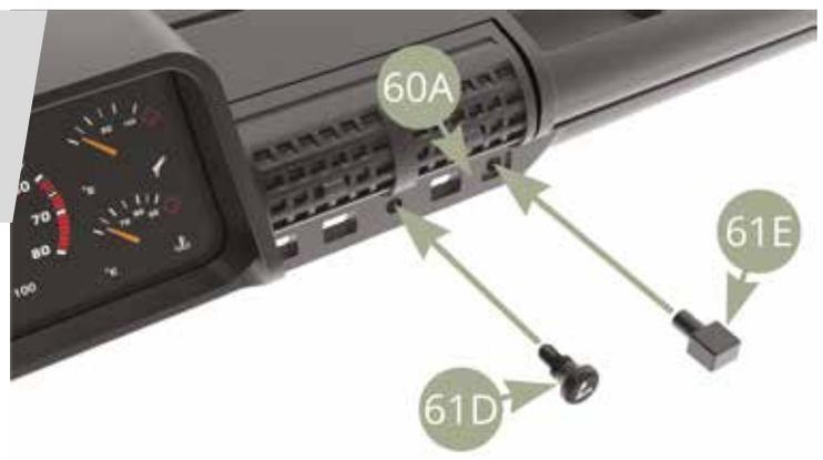
61D Cigar lighter and 61E Optional button plug installed on 60A Upper dashboard panel.
