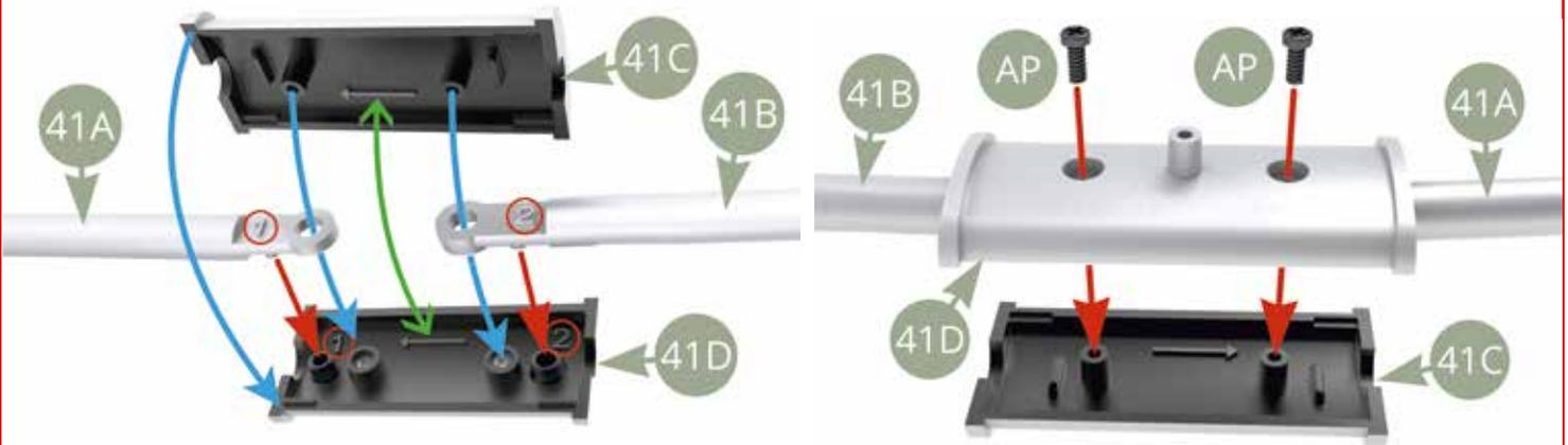
Pre assembled Catalytic converter and Exhaust pipes.
