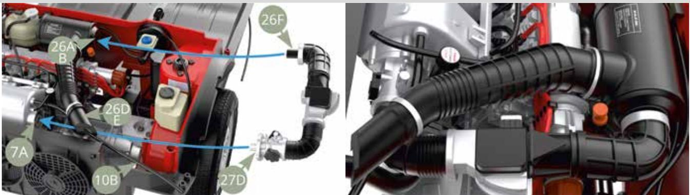
Fit 7C Vacuum hose to 27D Throttle body nozzle.
