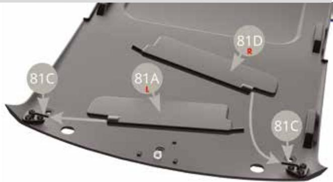
Fit 81F Interior lamp into 81E Lamp housing. Fit 81E Lamp housing to 80A Ceiling panel, engaging also 81D Right and 81A Left Sun visors' pivot pins.
