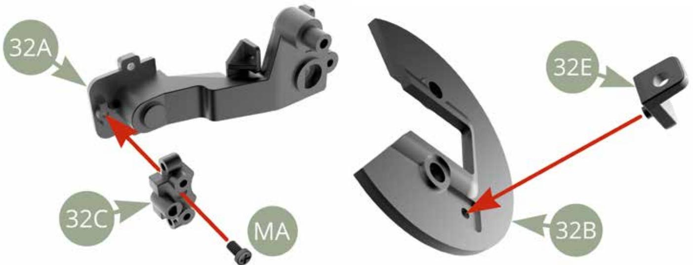
Slide 32B Brake dust shield to 32A Rear axle left trailing arm, aligning and fixing with two AM screws.
