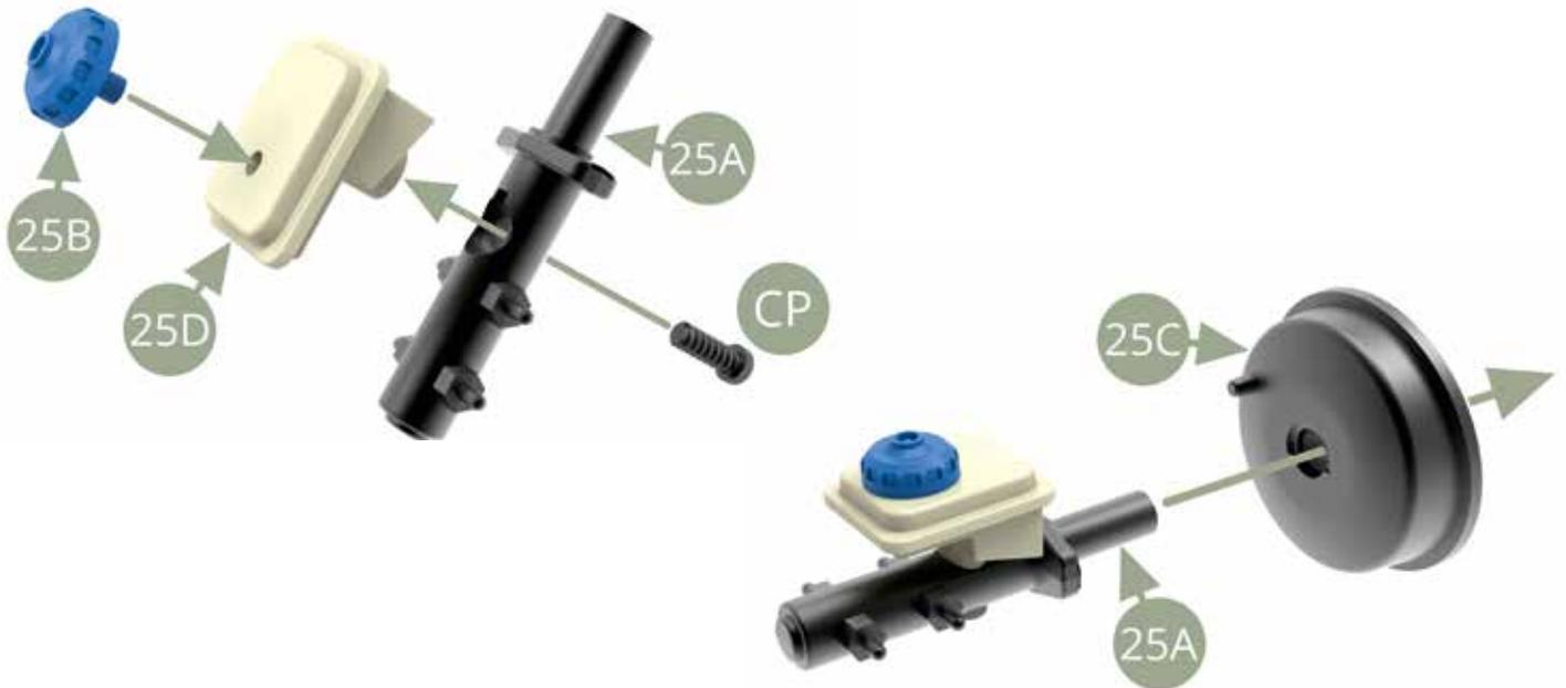
Fit 25A Brakes master cylinder to 23A Firewall and fix with CP screw.
