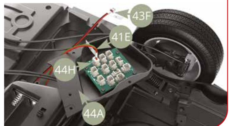
43F Battery compartment cable A (red - black) plugged into Nest A of 44H Circuit board.
