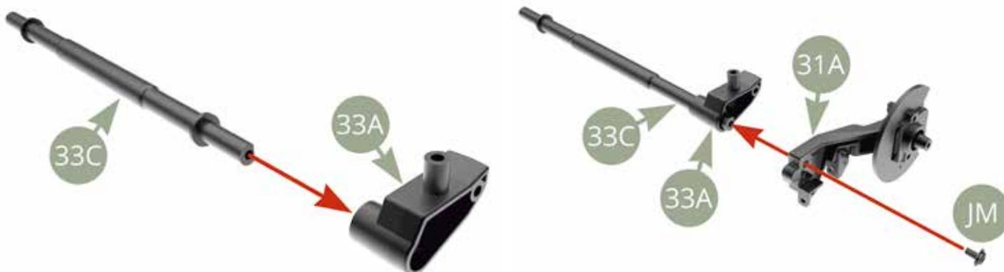
Fit 33D Rear torsion bar to 33A Rear axle left mount.
