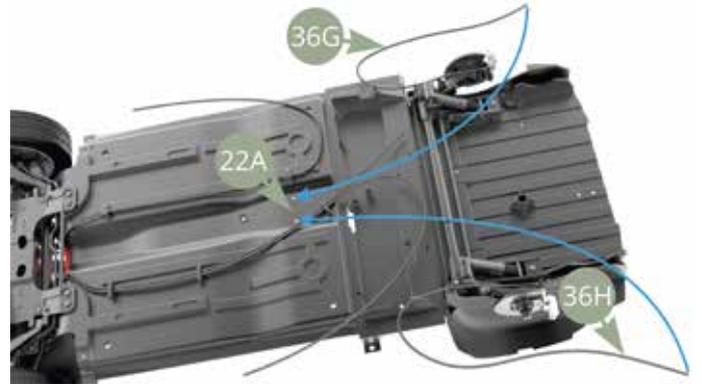
Note 36G Left and 36H Right parking brake cables fit through respective holes in 22A Chassis panel. 36G Left and 36H Right parking brake cables exiting on upper side of 22A Chassis panel.
