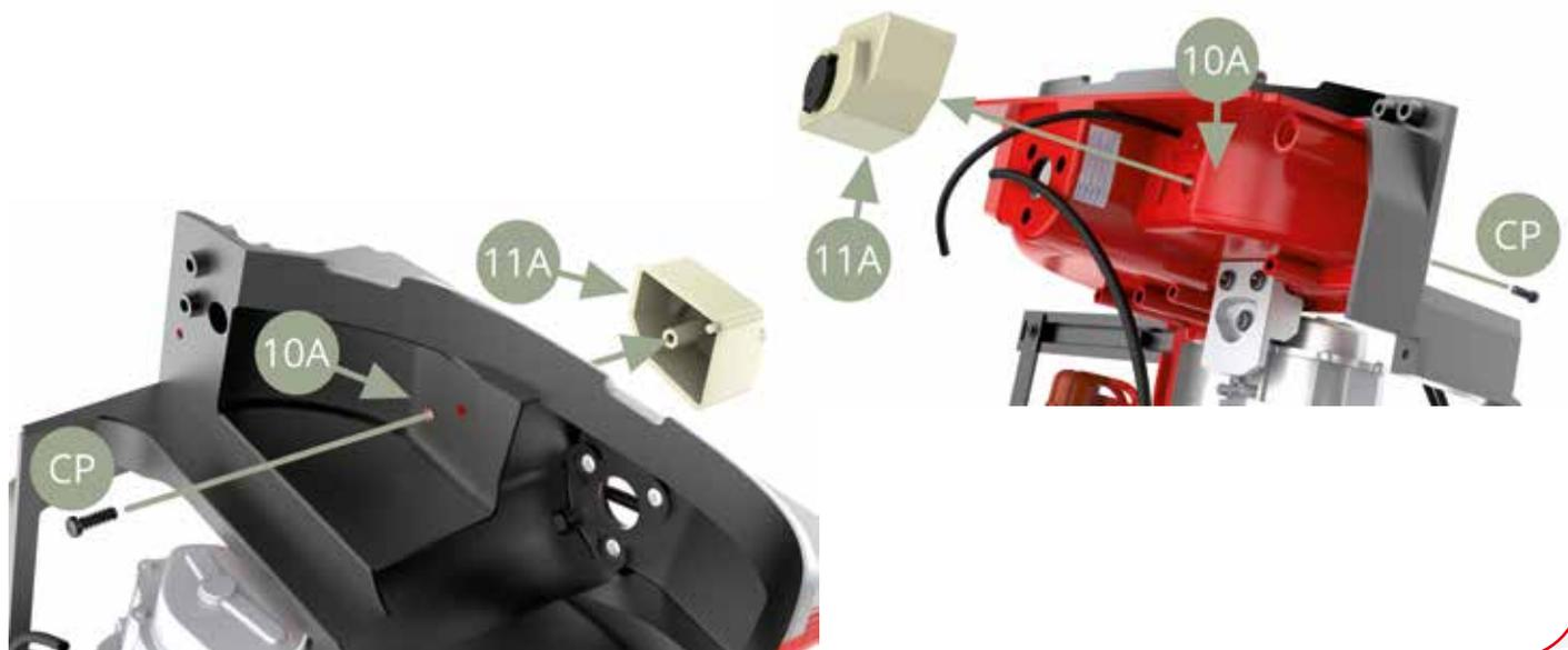
Installed 11A Washer fluid reservoir.
