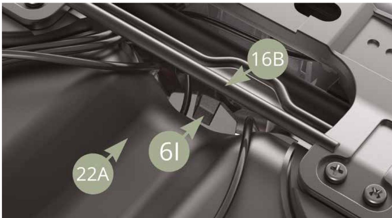
Note 6I Exhaust manifold flange niche and fit 41A Front pipe end into it, passing down under 16B Subframe bar (top and bottom illustrations).
