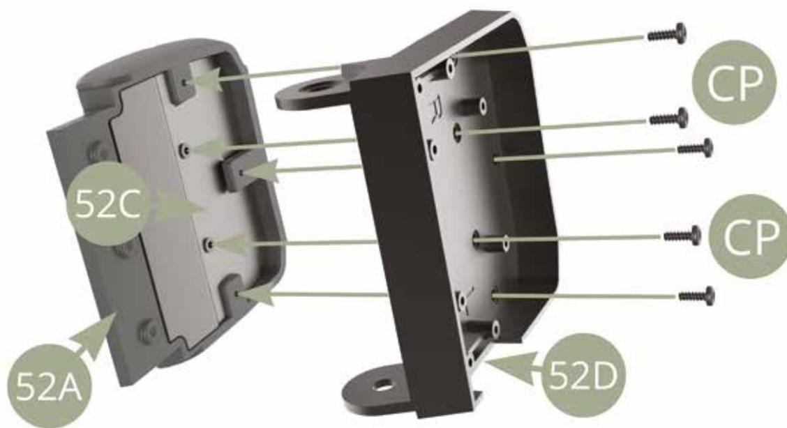
Fix 52A Front left seat cushion to 52D Front left seat base with three FP screws.
