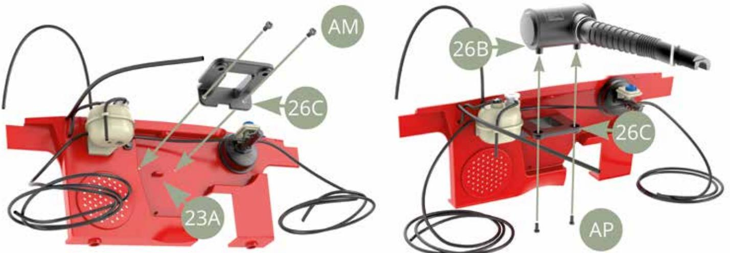
Prior to installation of pre assembled 23A Firewall to Engine compartment, and for further assembly convenience, identify : 8I Heater pipe, 24H Coolant hose, 12G and 14G Brake fluid pipes.
