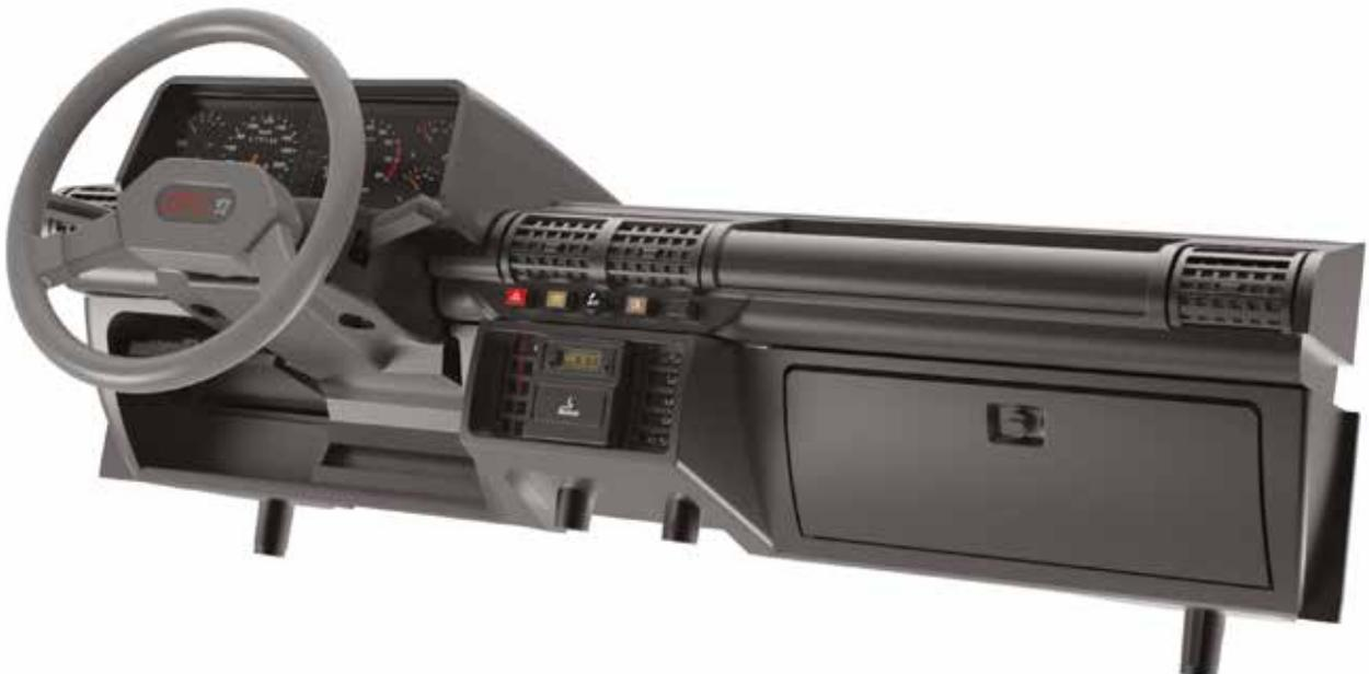
Fit 48A Centre console to 62A Facia panel and fix with two AP screws.
