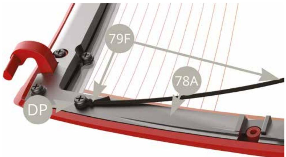
Fit DP screw to upper left corner of 78A Tailgate inner panel, leaving space under screw head to loop over and tie to knot second 79F Rear shelf support rope (lower illustrations).
