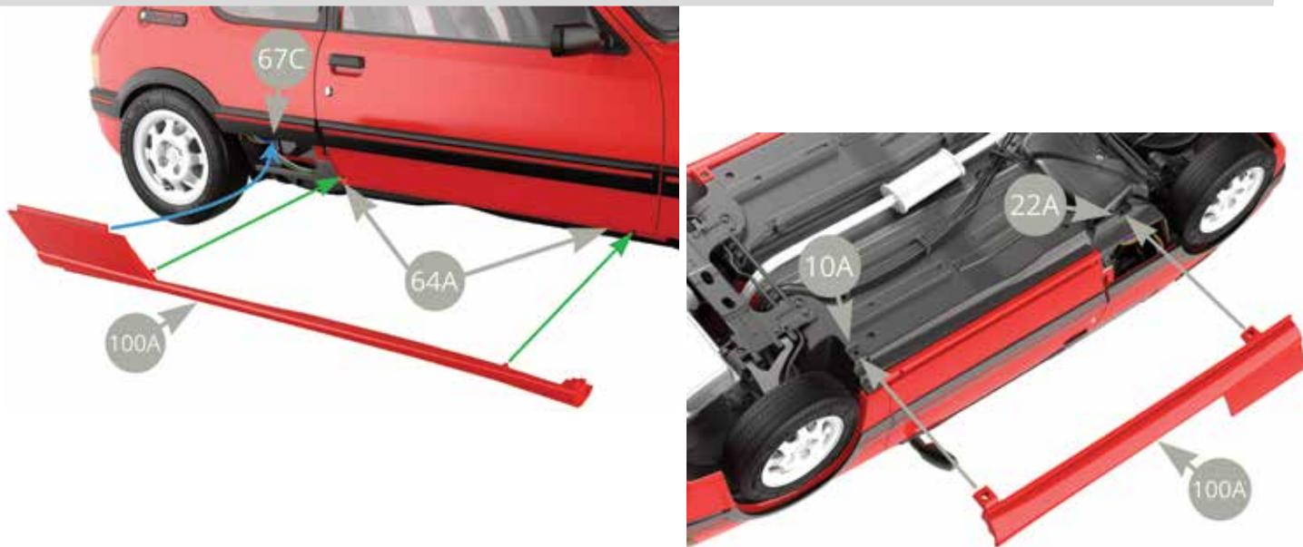
Fix 100A Right lower panel to 22A Chassis panel and 10A Front frame with two BM screws.
