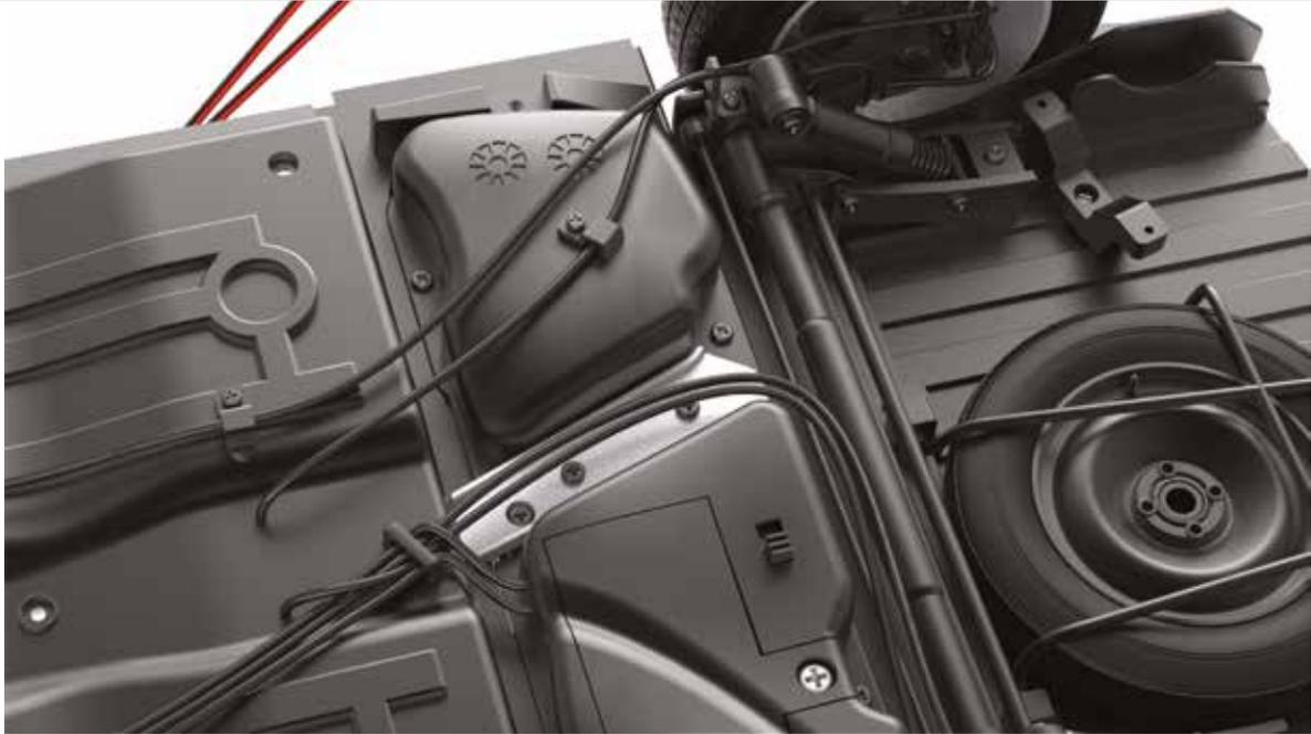
Prior to installing the Exhaust duct, take note of first two attachment points : 41A Front pipe goes under 16B Subframe bar (further explained on next two illustrations) and 41D Catalytic converter top peg fits into 22A Chassis panel nest.
