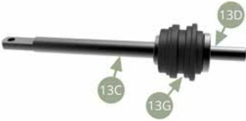
Fit 13F Rubber bellows onto 13C Driveshaft.
