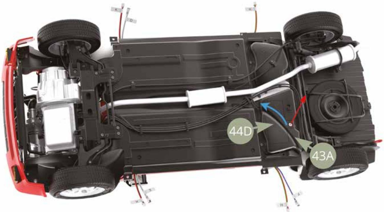
Fit two AAA size batteries into 43F Battery compartment of Right side Fuel tank, observing "+" and "-" polarities (green arrows). Put ON battery compartment switch (red arrow). Re-close Battery compartment.
