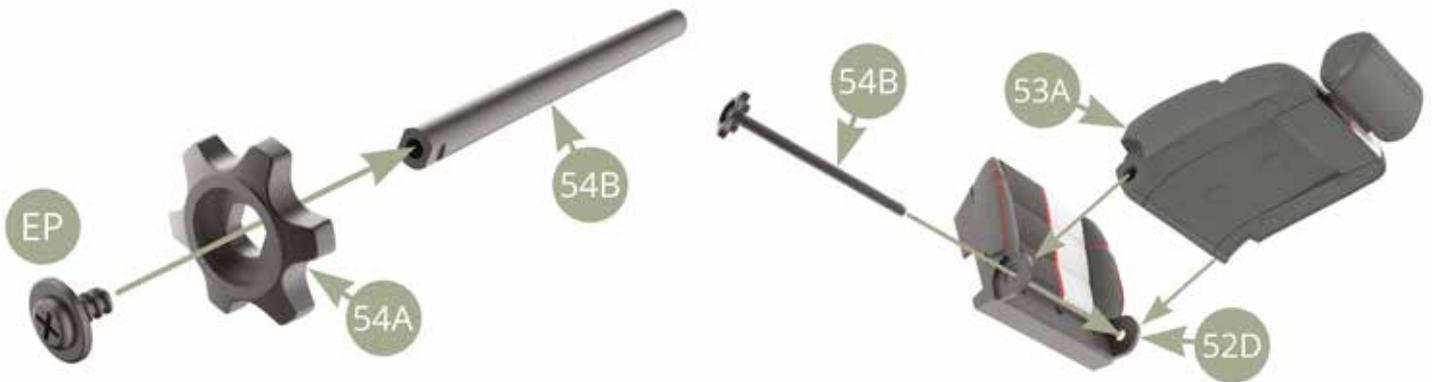
Fit 54A Backrest adjustment wheel to the other end of 54B Axle and fix with EP screw.
