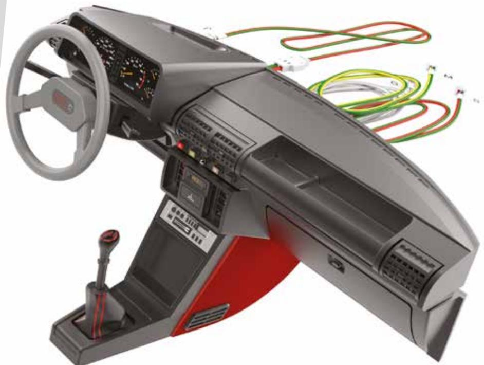
Fit 45A Saloon floor to 48A Centre console with 62A Facia panel and fix respectively with three and two AP screws.
