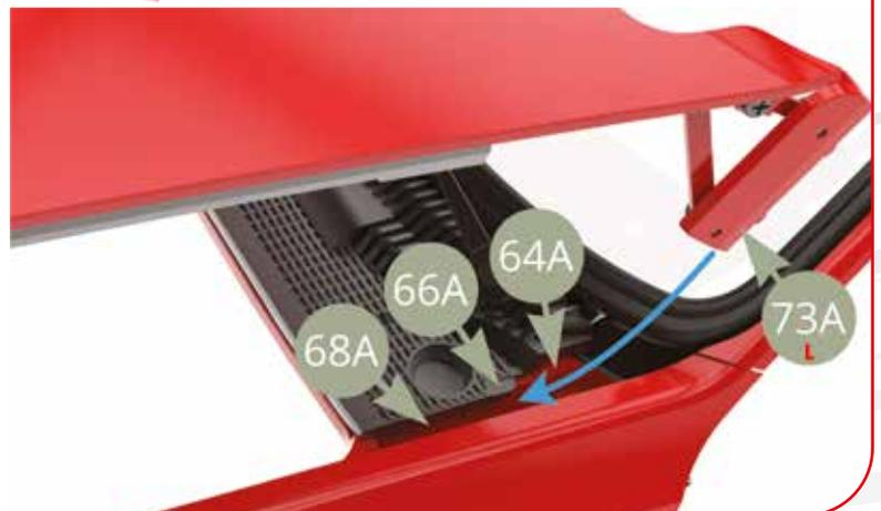
Make sure 1A Bonnet is pressed home flush with adjacent surfaces. Turn car body over, and fix 73E Right, 73A Left hinge bases to 64A Body frame and 68A Front subframe with four CM screws (lower illustrations).
