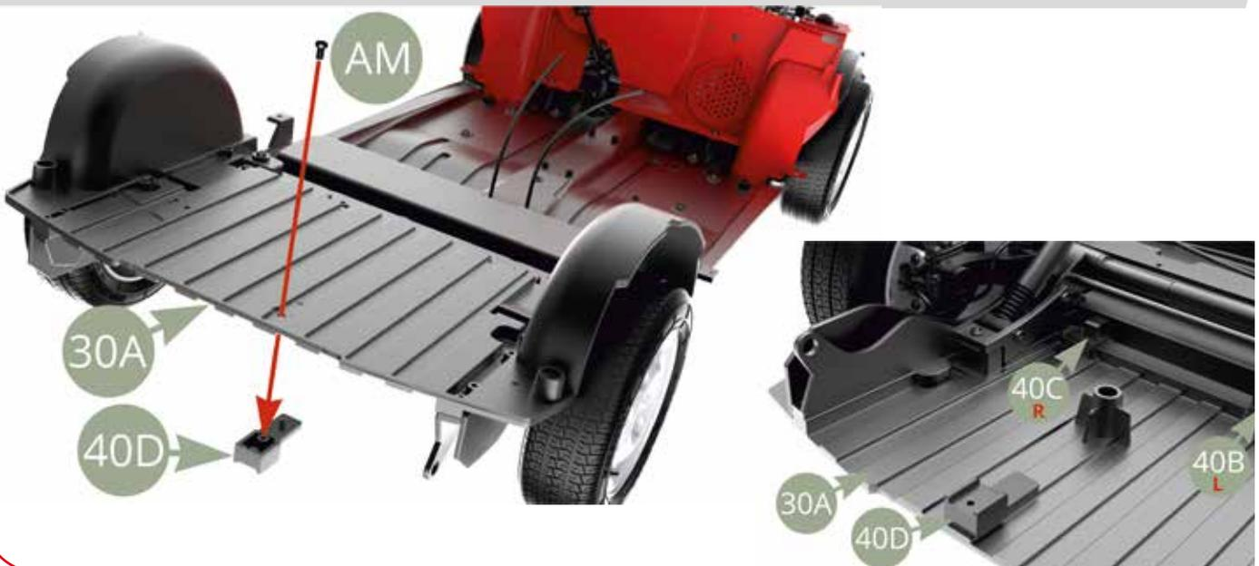
Fit, by carefully bending, 40A Spare tire holder legs into 40C Right and 40B Left spare tire holder shoes holes.
