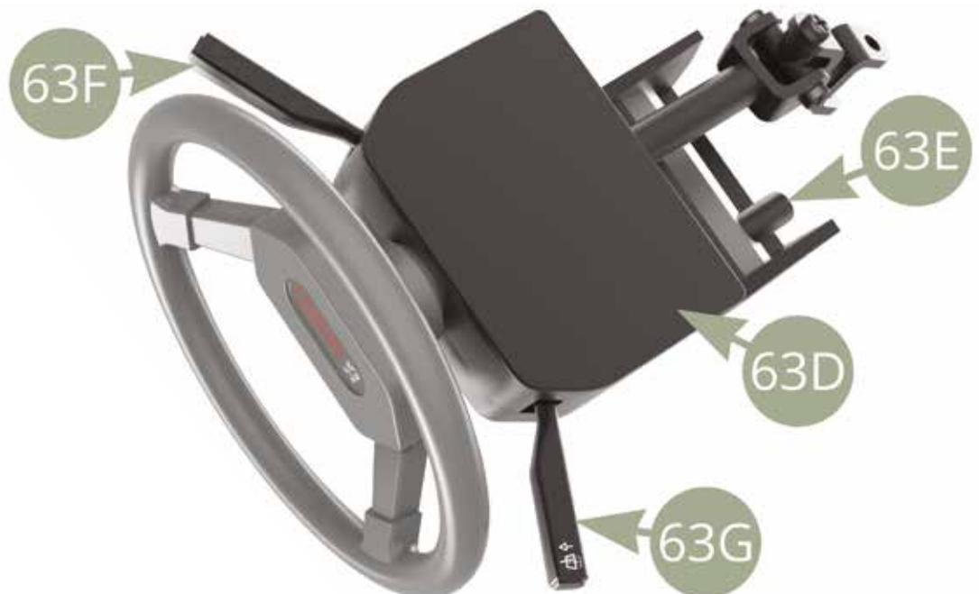
Fit 63E Steering column lower housing to 62A Facia panel and fix with two BM screws (upper and lower illustrations).
