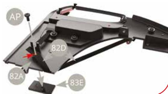
Lower end of 82D Rear left safety belt is attached. Pull to tighten the upper end of 82D Rear left safety belt (blue arrow).
