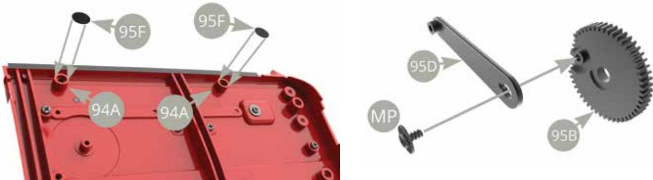
Fit 95B Big gear to 94A Right door inner panel and fix with MP screw. Fit 95A Right door glass with its two guiding tabs to the uppermost position (blue arrows) into the grooves of 94A Right door inner panel, and fix it to raised 95D Lever with MP screw.
