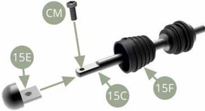
Slide 15F Rubber bellows along 15C Driveshaft to cover the joint (blue arrows motion).
