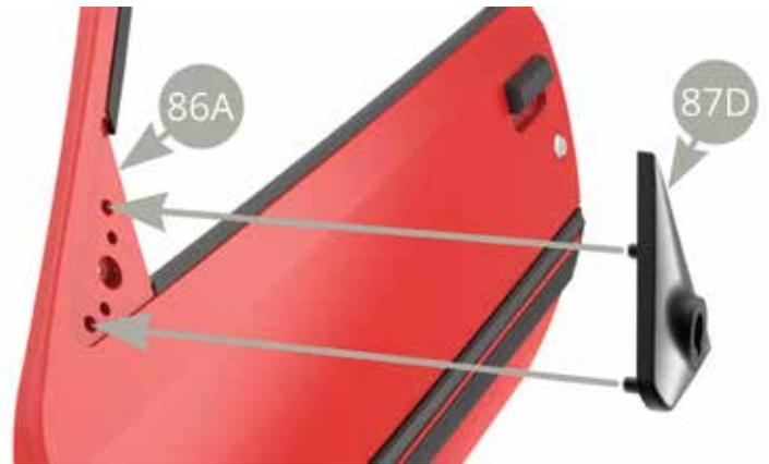
Fit 87C Side mirror housing to 87D Side mirror base and fix to 86A Left door from its inner side with AP screw (lower illustrations).
