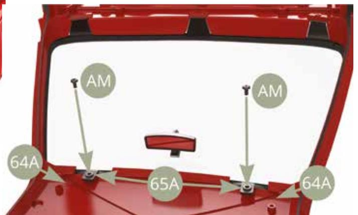
Windscreen with Inner Rear-view mirror is installed to Body frame.
