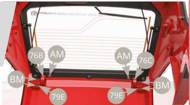
Check opening and closing of 64A Tailgate. Adjust tension of four BM screws (previous illustration) if needed for smooth work of hinges.
