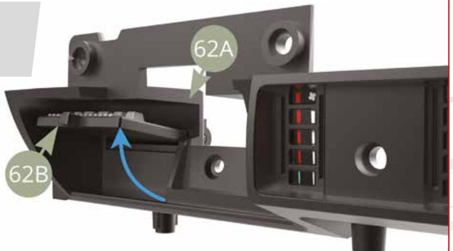
Fit 62A Facia panel to 60A Upper dashboard panel and fix with four AP screws.
