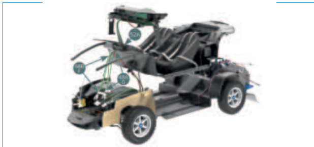
Step 4 Position the dashboard (3A) on the cabin floor (62A) and secure with two IP screws.
