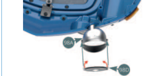
Step 3 The cover with beam guide (98D) is attached to the right fog light housing (98A).
