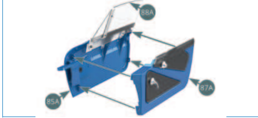
Step 7 Attach the right inner door panel (87B) to the right outer door panel (87A) with two ZM screws at the front (illustration above) and two ZM screws at the rear (illustration below).
