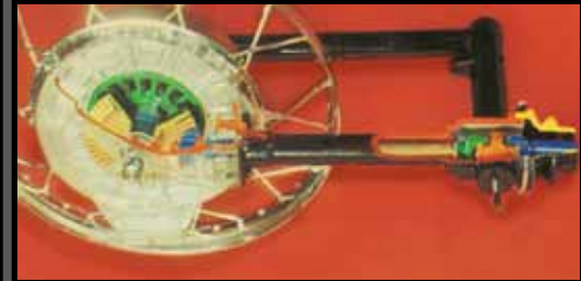
Rear fork, transmission, shaft, pinion and crown-gear, double joint
