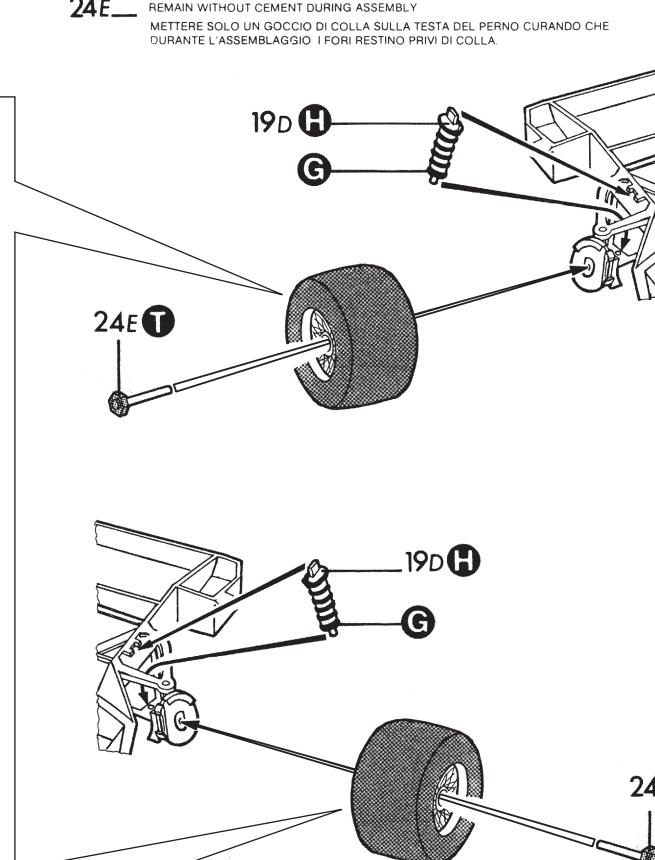
**24E**— JUST PUT A DROP OF CEMENT ON THE PIN HEAD MAKING SURE THAT THE HOLES REMAIN WITHOUT CEMENT DURING ASSEMBLY
