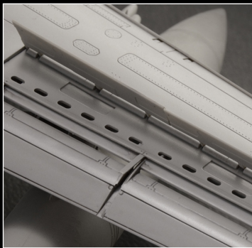
Retracted or extended flaps and slats Movable ailerons
