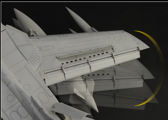
Movable variable geometry wings and wing pylons
