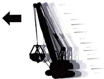
Forward by pushing both joystick to the front.
