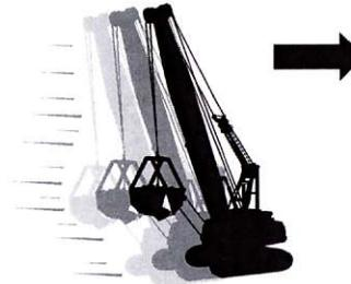
Backward by pushing both joystick to the back.
