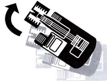
Right turn by pushing right joystick to front.
