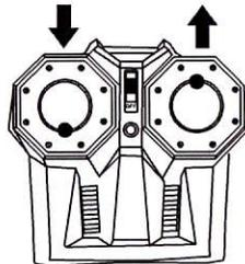
Left spin by pushing left joystick to front and right joystick to back.
