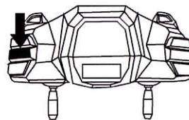
Latticed boom tilt up by pressing (L2) button.
