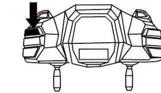
Releasing hoist rope by pressing (L3) button.
