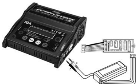
Connection diagram in the balance charging/storage/ discharge mode
