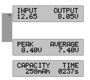
The next read-out relates to the working voltage of the charger, which always adjusts to the requirements of the connected battery. OUTPUT is somewhat higher than the current voltage level of the battery being charged.
