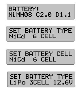
First appear the values of your last charging: type, number of cells, charge- and discharge current. At this screen you can turn the knob to enter the battery type, in this instance: NiCd. Any types compatible with the charger can be entered and confirmed by pressing the button. The number of cells then flashes and you can enter the appropriate number. Confirm by pressing the button.
