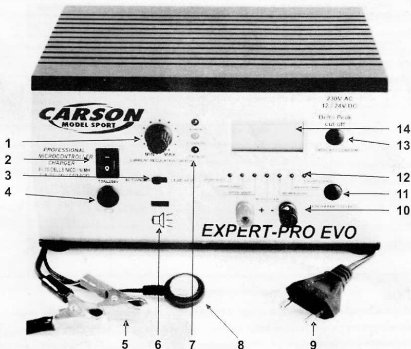
1. CHARGING CURRENT ADJUST SWITCH – adjusts the level of charging current
