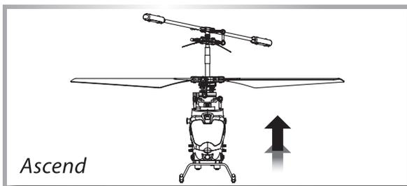
When you push up the left stick (throttle) the speed of the main rotor blade will increase and the helicopter will go up.
