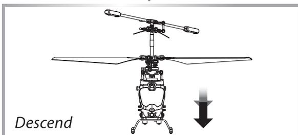
When you pull down the left stick (throttle), the speed of the main rotor blades will decrease and the helicopter will go down.
