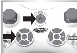
**RESET function:** Press the button B and turn ON the transmitter
