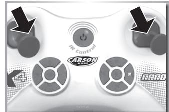
**Calibration function:** If the quadcopter drifting always to one side after start, you should bind the 2.4 GHz signal again and you must put the model on a horizontal surface (table, floor).
