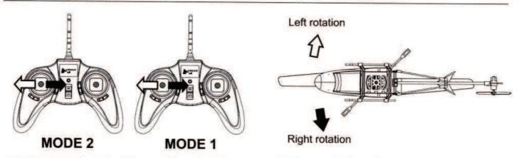
Rudder (Collective Torque Yaw) rotates your helicopter's fuselage Left / Right
