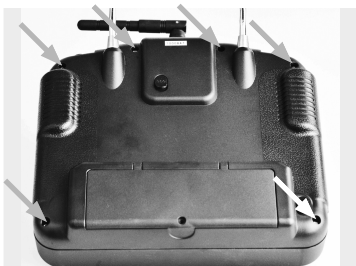
Open the cover of the transmitter by unscrewing the 6 screws. See picture.
