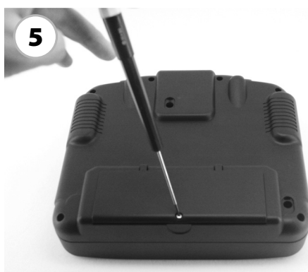
Replace the battery box.
