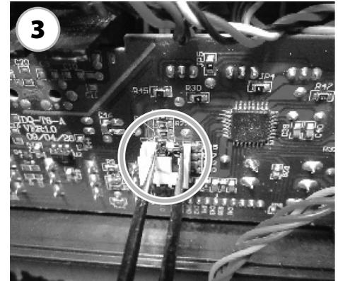
3. Find out the 3 PIN terminal, and plug the jumper wire in the location of the 2 PIN terminal.
