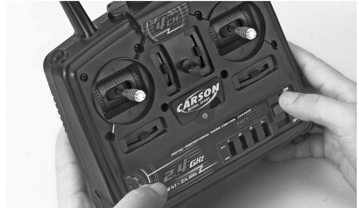
4. Press the frequency bind button again to get it rebound. The transmitter gets into normal working mode again.
