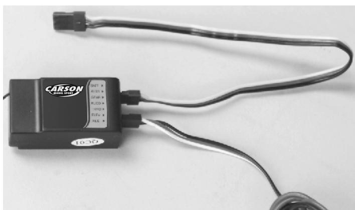
5. Disconnect the binding plug again. The LED will remain lit for a few seconds. The RC system will revert to normal operation.
