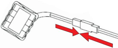
**Connect the battery to the model. The LEDs will flash. If the big LED will be lights continuously, the receiver is in binding-mode. Now you can loose the binding-button.**
