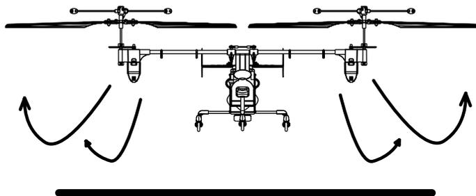
For this reason the flight behaviour of the model at low heights is rather unstable. If the restless flight behaviour causes difficulties for you, increase the flying height by degrees.
