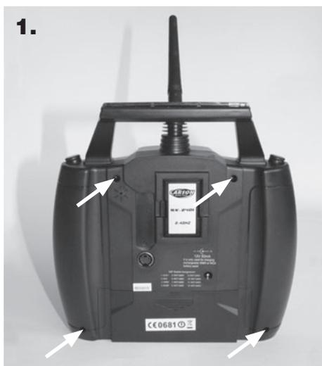
1. Unscrew the screws in the transmitter cover, shown as the picture.
