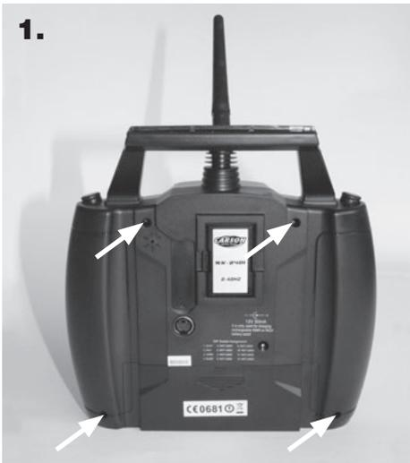
1. Unscrew the screws in the transmitter cover, shown as the picture.
