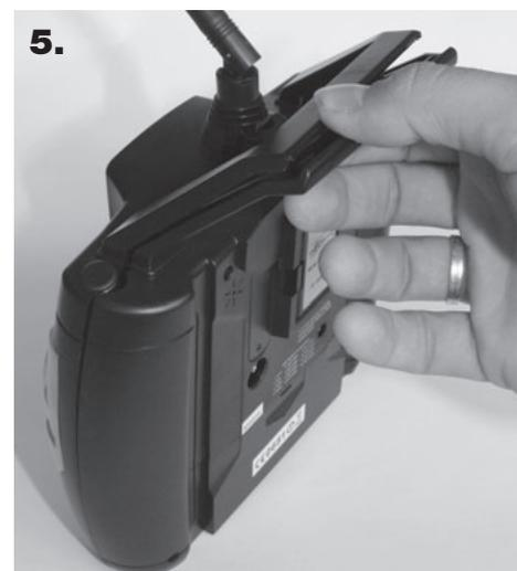
5. Pull in the pin D. Mount the rear cover and tighten the screws, and move the throttle trim to the lowest position. the switch process is finished.
