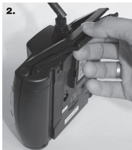
2. Slightly separate the rear cover from the front one of the transmitter.
