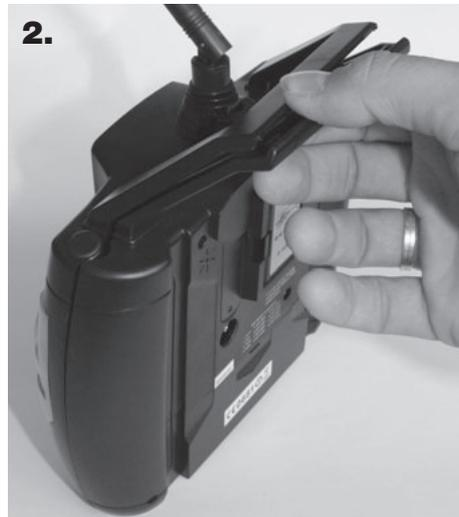
2. Slightly separate the rear cover from the front one of the transmitter.
