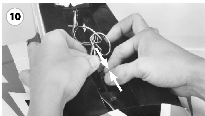
Connect the Y cable (Aileron connections).
