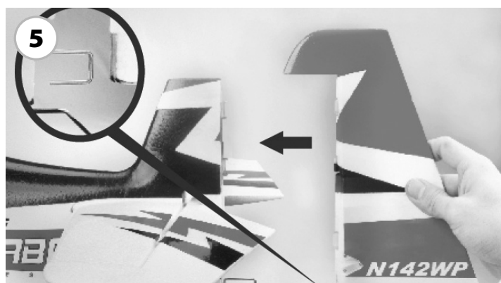
Install the Rudder.
