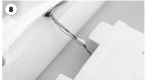
Connect Aileron servo electrical wire (3CH exception).
