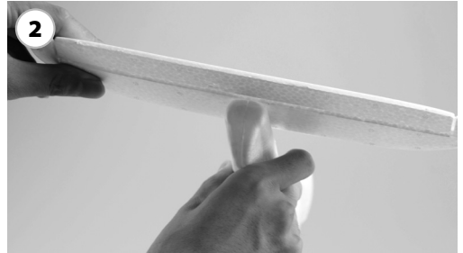
The tailplane bonding to the body firmly
