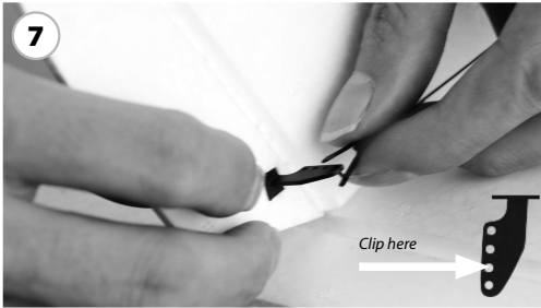
Connect the servo rod to the Rudder servo horn.
