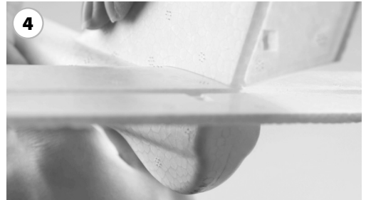
Bonding the fin to the body firmly
