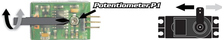
Now switch on the transmitter and check to see whether the servo can be operated with the joystick as normal. After a (simulated) loss of reception caused by switching it off, the servo should operate in its emergency position.
