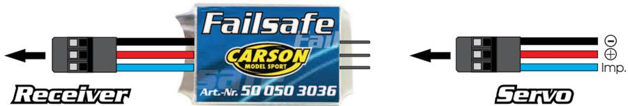
A 3-pole cable (servo cable) with a plug that fits your receiving unit is soldered on at the "+", "-", and "Signal" input observing the correct polarity. There is a corresponding female cable socket at the output.
