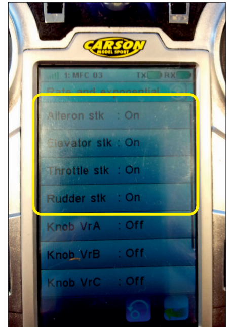
12: At the end of programming it must be enabled on all channels (1-4) (set to ON) be.
