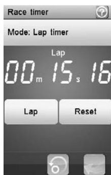
In this example, the lap button was just touched and the last lap time is displayed for 3 seconds.
