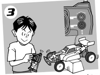
Put the RC car on a box or some type of stand and check if it works fine. If tire rotating does not stop, adjust throttle trim.
