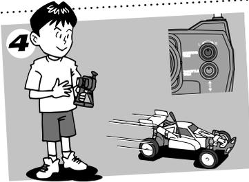
Let the RC car run slowly without controlling the steering wheel. If the RC car does not run straight, adjust the steering trim.
