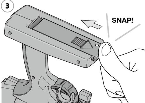
Make sure the battery was installed correctly and close battery cover.
