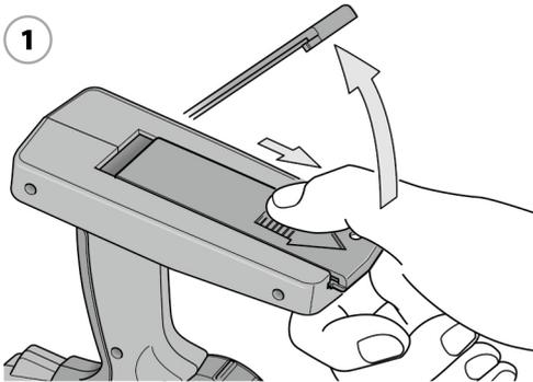
Slide battery cover to indicated direction and open it. Install new battery (Note polarity).
