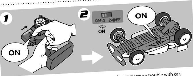
Switch on the transmitter first, then switch on the RC car. Make sure to follow this order when turning on your RC car. Performing the wrong
