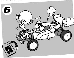
**6** Avoid continuous running. Allow the motor to cool down approximately 30 minutes after running.
