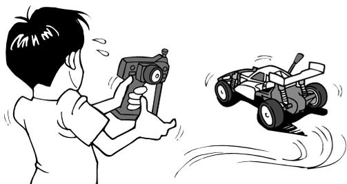
When the RC car does not run straight, adjust the steering trim. Let the car run without touching the steering wheel to check the direction and
