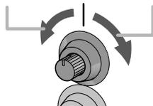
adjust by turning the steering trim knob to the opposite direction the RC car naturally goes.
