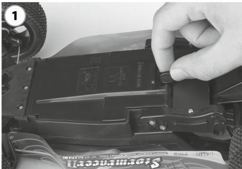
Turn knob at the bottom side of the chassis toward the indicated direction and open the battery cover.
