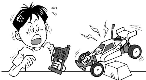
If the RC car moves on its own accord when throttle trigger is in neutral, adjust the throttle trim. Turn knob into position till the tires of the RC car stop rotation.
