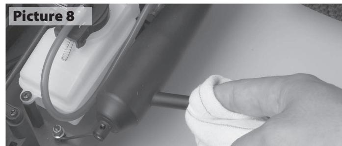
Then apply after run oil through the carburettor, and pull the pull-start a few times to get it through the engine. This is recommended if you plan on storing the car for more than a day. Methanol evaporates in water and can cause internal corrosion to engine parts. It is always a good idea to check all the screws, nuts, and bolts before and after each period of racing.
