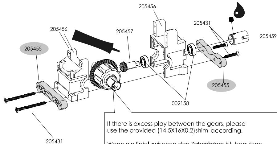
If there is excess play between the gears, please use the provided (14.5x16x0.2) shim according.
