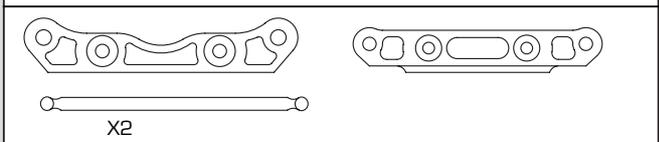
**205508** Rear lower suspension mounts (Aluminum) with pin (Toe in 2°)
