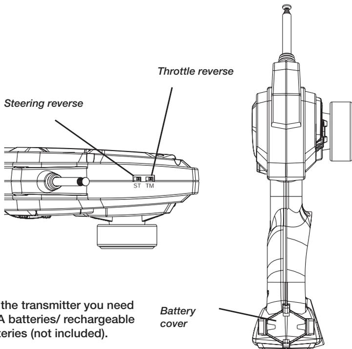
For the transmitter you need 8 AA batteries/ rechargeable batteries (not included).
