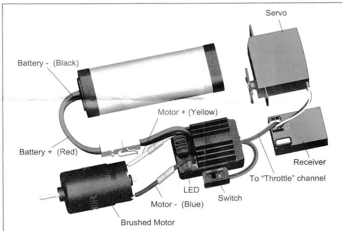
The control cable of the ESC (trio wires with black, red and white color) is connected to the throttle channel of the receiver (Usually CH2). The “Motor +” and “Motor –” wires are connected to ESC without any order. If the motor runs in the opposite direction, please swap these two wire connections.
