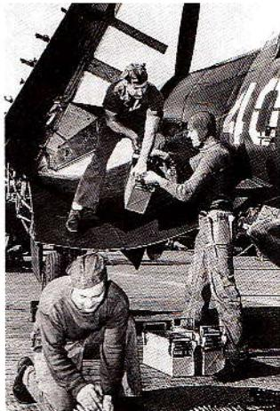
■ F4U-1~4 Corsairs during WWII standard armament was 6 12.7mm machine-guns with a total of 2300 rounds.
