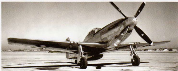
●エアロプロダクツ社製のプロペラを装備したP-51K。 The P-51K was equipped with an Aeroproducts propeller.
