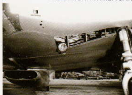
●脚収納庫に取り付けられた着陸灯。 前縁にはガンカメラが見える。 The landing light was installed in the main landing gear well. The gun camera can be seen in the wing leading edge.
