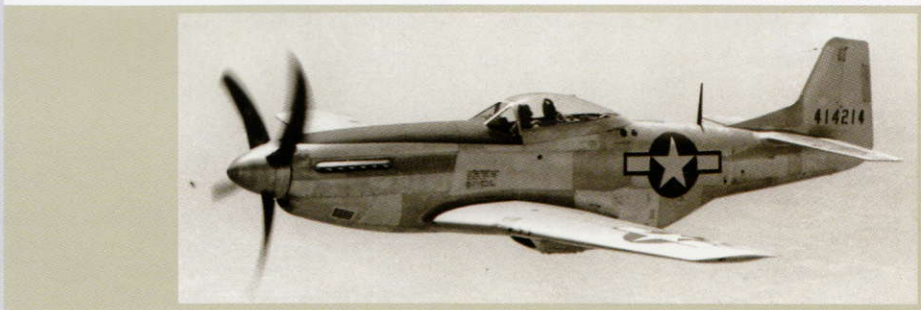
●水滴形キャノピーを採用し、武装を強化したP-51D。 The P-51D was equipped with a teardrop-shaped canopy and increased armament.
