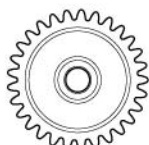
MA13 ×1 29Tピニオンギヤ 29T Pinion gear 29Z Motorritzel Pignon moteur 29 dents
