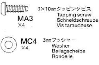
**《C12の取り付け》 / Attaching (C12) / Einbau (C12) / Fixation (C12)**
