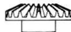
MB4 ベベルギヤー(大) Large bevel gear Kegelrad groß Grand pignon conique
