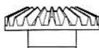
MA7.....×2 50602 べベルギヤ(大) Large bevel gear Kegelrad groß Grand pignon conique
