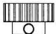
SA1 21Tピニオン……………×1 21T Pinion gear 21Z Motorritzel Pignon moteur 21 dents
