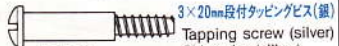
BB2.....×4 3×20mm 段付タッピングビス(銀) 2090017 Tapping screw (silver) Schraube (silber) Vis (argent)
