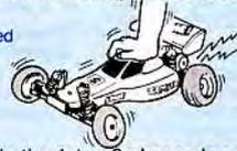
Driving for long periods in the 1st or 2nd speeds can also burn out the resistor.
