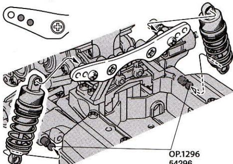
★Attachment points vary according to damper position. Attach Item 54296 M-06 3x34mm Titanium Coated Ball-Head Suspension Shaft to lower arms when using middle or innermost holes on damper stay.
