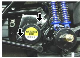
Take off motor cover by removing screws marked by arrows.
