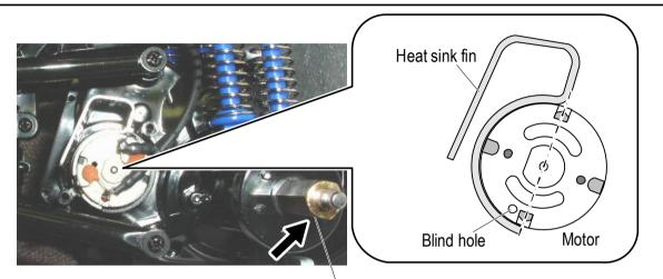
Install the motor, aligning openings as shown in illustration.
