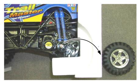
Use box wrench to remove central nut of right-rear wheel. Remove wheel.
