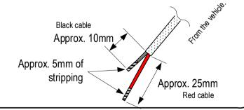
Strip the sleeve off from the cable as shown.
