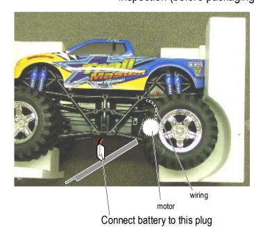
Insert battery on underside of chassis, operate transmitter and check rotation of back wheels.
