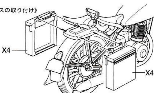
●DKW NZ 350 medium cycles were mainly used as courier cycles. The late version was equipped with a small head light and metal carrying cases.
