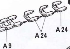
Fix Track to Sprocket first.
