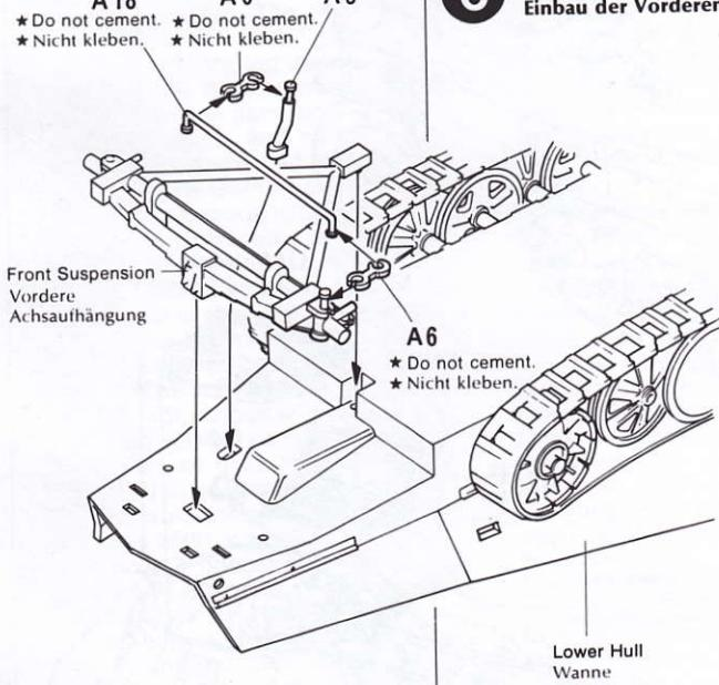
**6** Fixing of Front Suspension
