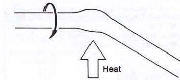
Heat a length of sprue. When melted a little, stop heating and pull to stretch it. Hold for about 15 seconds to cool and cut to proper length.
