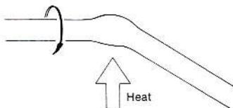
Heat a length of sprue. When melted a little, stop heating and pull to stretch it. Hold for about 15 seconds to cool and cut to proper length.
