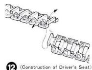
Rear seat differs according as the vehicle is fighting or running. In fighting, the rear seat is folded up so that the machine gun can be swivelled.
