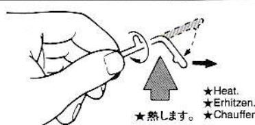
★Heat sprue as shown. Remove from heat and stretch. Allow to cool and cut to required length.
