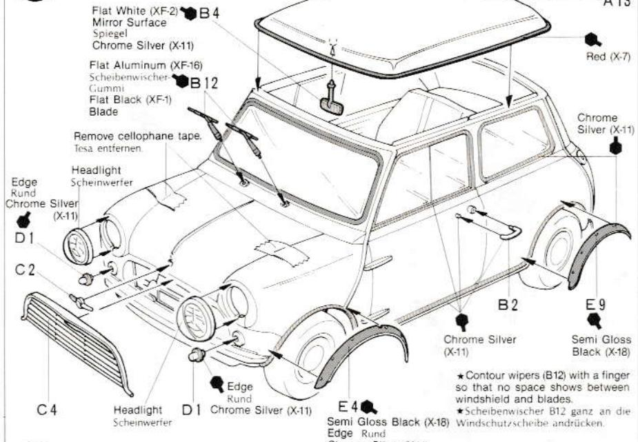
★ Contour wipers (B12) with a finger so that no space shows between windshield and blades.
