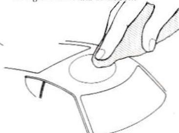
decal down with a steamed towel so that the warmed, wet decal will fit the surface well. Cut off the excess transparent portion around a decal before applying. When so done, you can expect a sharp finish with the decal precisely in its specified place.
