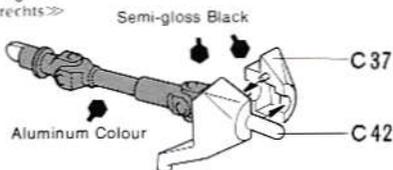
**5** Construction of Gear Box B
