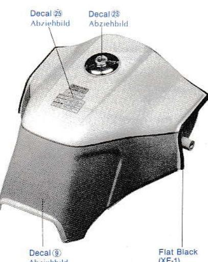
**34** Assembly of Fuel Tank
