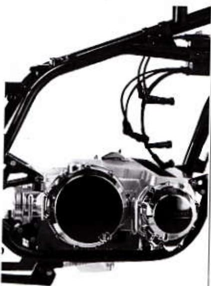
**5** Placing Crank Case into Frame
